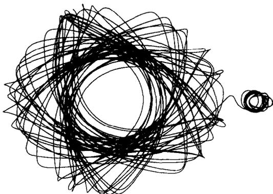
Fig. 3. A configuration space plot  $(x, y)$  of the 58 iterate chaotic transfer to the Moon. The final state at  $b$  is a precessing ellipse around the Moon corresponding to the targeted invariant torus.
