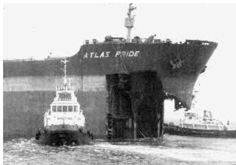
FIGURE 5.1.5. Bow damage to Atlas Pride.
