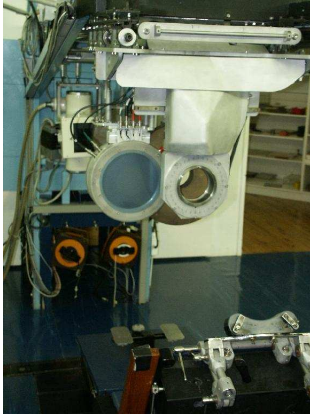
FIGURE 6.2.2. The exit of the proton beam from the cyclotron at IThemba Labs.
