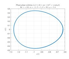
Plotting both the full parametric solution and the tail of the solution, we see that the full solution appears to exhibit very strange and unpredictable behavior. However, once the end behavior of the solution is examined more closely we see that the solution approaches a single orbit with period  $T=2\pi/\omega$ .
