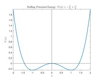
We can see from the plot that the positions of the minimum values of the potential occur at  $x=\pm 1$  and take the values  $V(x=\pm 1)=-\frac{1}{4}$ .
