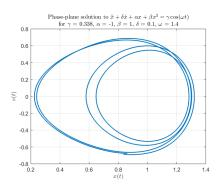
Further increasing the magnitude of the driving force and the length of the t interval reveals the same pattern of behavior as in the previous two cases. In this case, the end behavior of the
