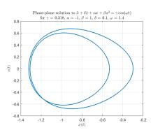
Increasing both the magnitude of the driving force and the interval t over which the solution is computed, we see phenomena similar to those in the previous solution plots. The initial behavior of the solution is unpredictable but the end behavior of the solution approaches a simple curve that is composed of two nested orbits. This demonstrates "period doubling" in the solution (wherein the period of the solution is  $T = 4\pi/\omega$ ).
