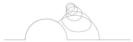
Figure 9. Vortex rings trailing the sphere, with  $\kappa=5$ . Values of  $\alpha$  are 0, -.1, -.59, -1.04 and -1.43
