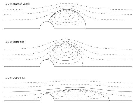
FIGURE 1. Examples of the three types of vortices obtained. The boundary of the vortex support, the streamline  $\psi = \alpha$ , is shown by a solid line. Other flow lines are dashed. The flow is from left to right in the far-field.  $\psi = 0$  on the axis and the boundary of the sphere. For all three flows  $\omega = 1$ . Values of  $\alpha$  are 0, -.6 and .47 respectively.
