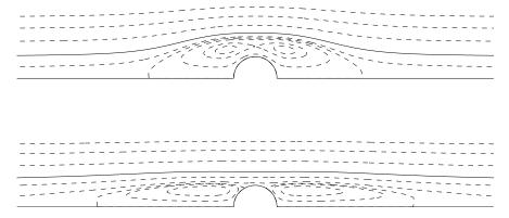
Figure 18. Streamline plots for vortices in the family given in Figure 16, for  $\alpha$  equal to .4 (upper plot) and .49.
