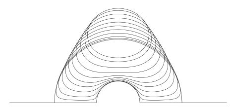
FIGURE 11. Vortex rings perturbed off the concentric spherical attached vortex, with  $\kappa=15$ . Values of  $\alpha$  are 0, -.005, -.03, -.1, -.22, -.36, -.6, -1, -1.6, -2.4, -3.
