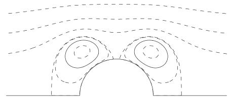
FIGURE 14. Streamline plot for flow with  $\kappa = 8$  with vortex regions near the end of the family shown in Figure 13. The stagnation points are near the top of the circle.
