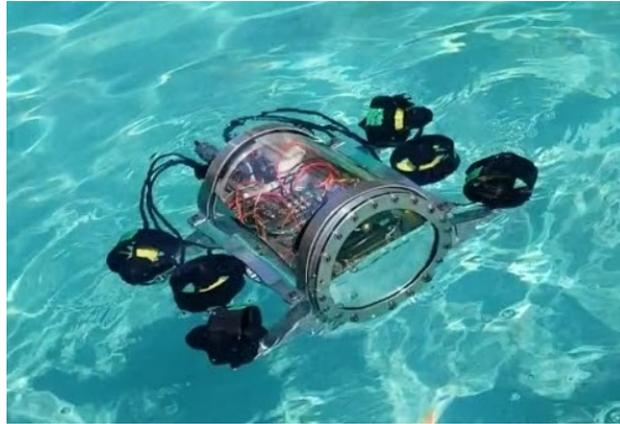
Figure 31: First Full System Leak Test
