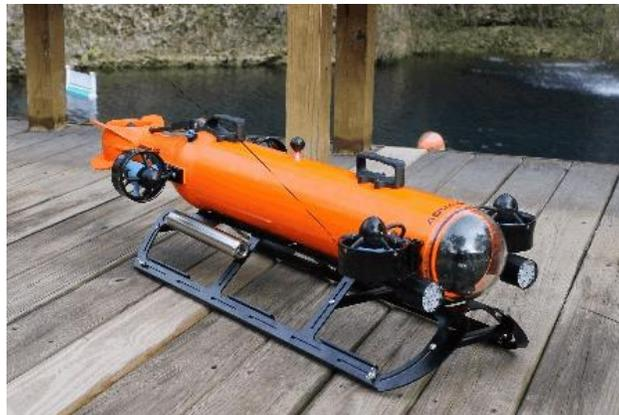
Figure 9: Example of Non-Torpedo AUV with Gimbaling Motors<sup>[22]</sup>
