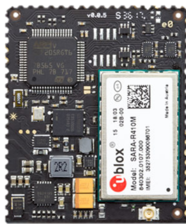
Figure 58. Example Cellular Communication Hardware
