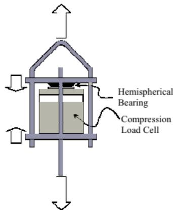
Figure 120: Compression Load Cell with Adaptor Diagram
