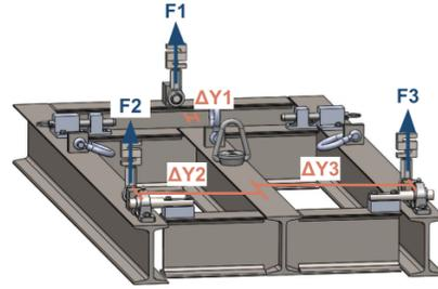
Figure 9: Load Cell Alignment Geometry - Y
