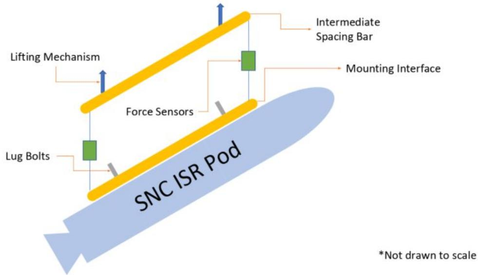
Figure 112: Parallel Plate Tilting Mechanism
