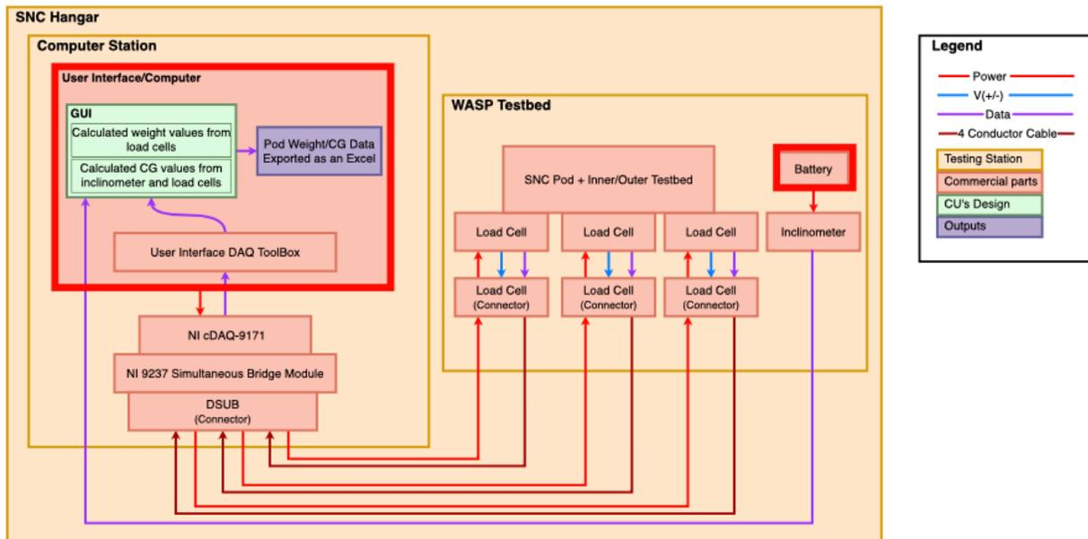
Figure 28: Functional Block Diagram of the Electronics
