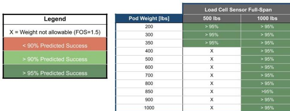
Figure 31: Load Cell Solution Space - CDR
