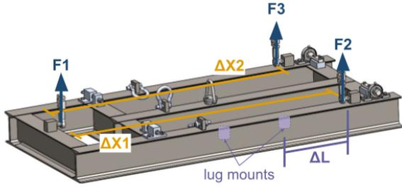
Figure 8: Load Cell Alignment Geometry - X
