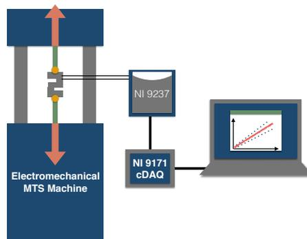
Figure 55: Load Cell Characterization Test Setup
