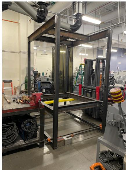
Figure 46: WASP Frame and Sliding Interface Being Assembled
