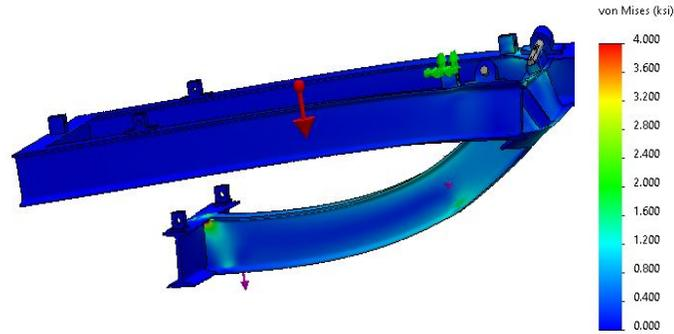
Figure 67: Testbed Assembly in Tilted Configuration Under 2205 lbs. of Load
