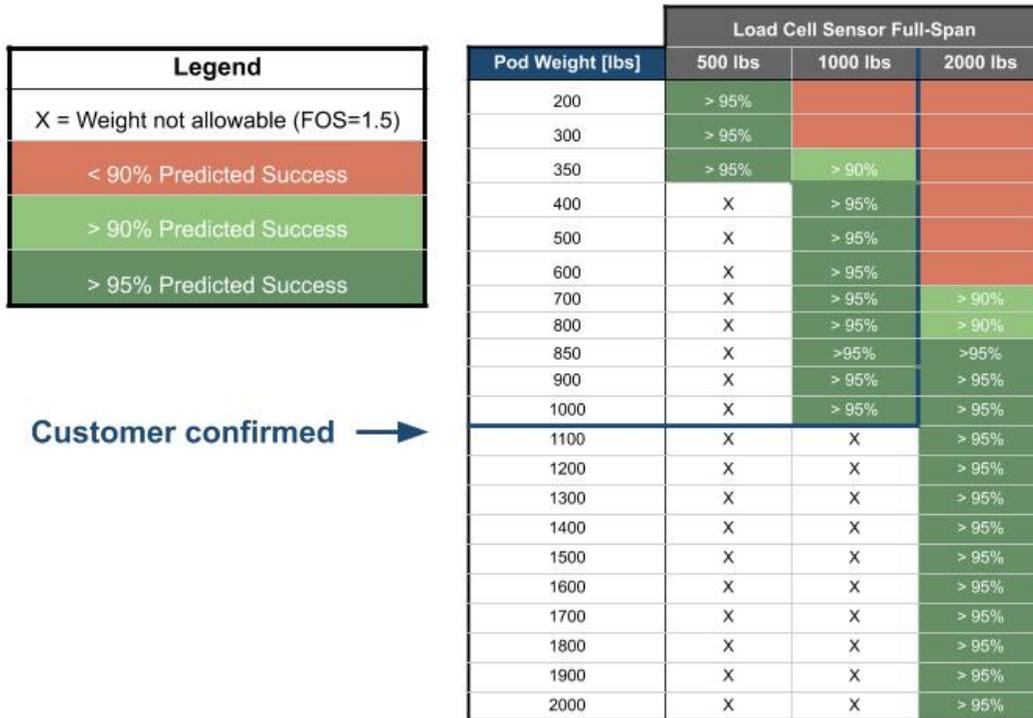
Figure 30: Load Cell Solution Space - PDR
