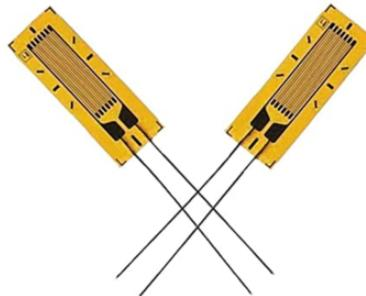
Figure 122: Strain Gauges
