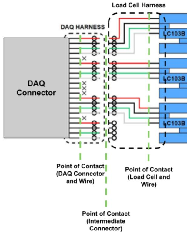
Figure 47: WASP Load Cell/Data Acquisition Harnessing
