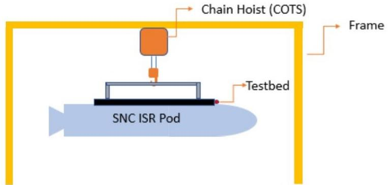
Figure 106: Chain Hoist Lifting Mechanism on WASP
