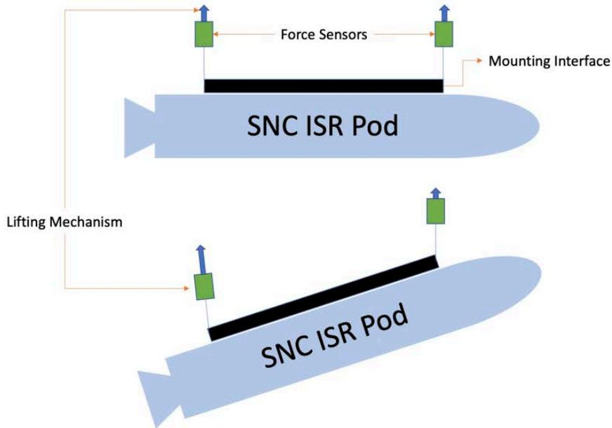
Figure 111: Suspended Testbed Tilting Mechanism
