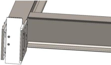
Figure 20: Plastic Plates used for Smooth Lifting
