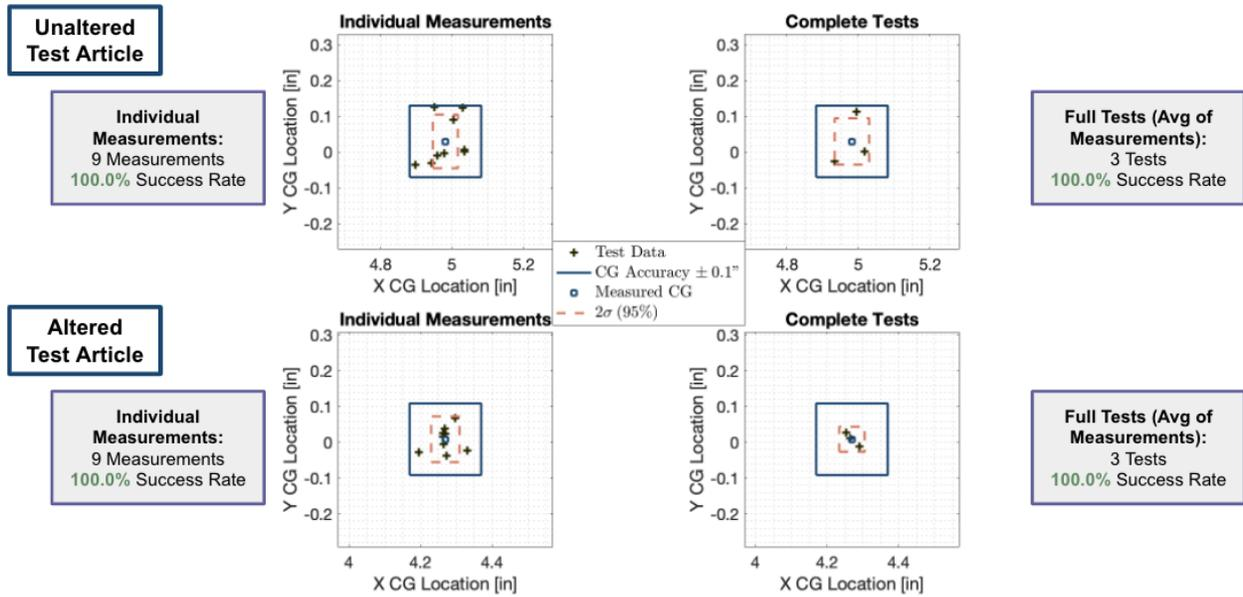
Figure 82: Predicted Range of X and Y CG Measurements for 95% of Individual Measurements and Tests
