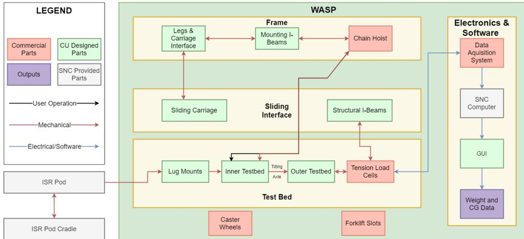
Figure 3: Functional Block Diagram for WASP
