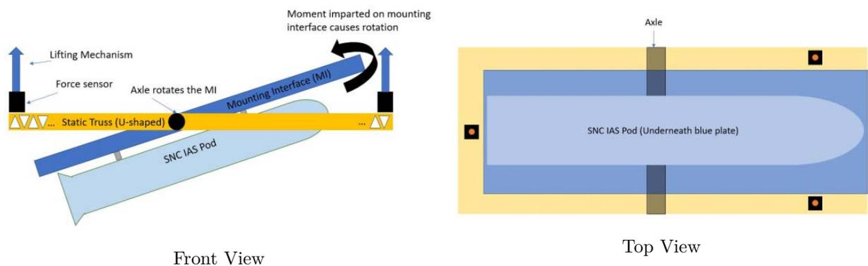
Figure 110: Axle-Based Tilting Mechanism
