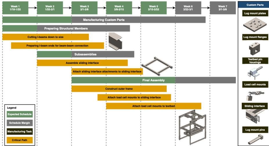
Figure 99: WASP Manufacturing Plan
