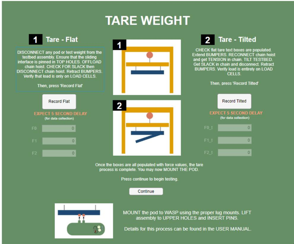
Figure 38: WASP GUI Tare Load Cells Menu
