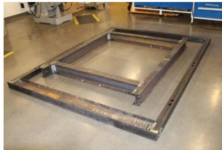
Figure 45: WASP Frame Side and Sliding Interface During Subassembly Stage
