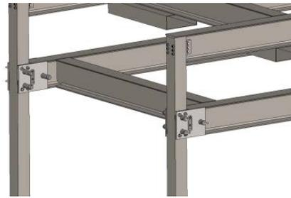
Figure 21: Sliding Interface Pinned to the Frame
