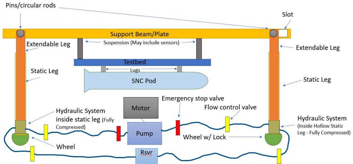
Figure 107: Hydraulic Lifting Mechanism on WASP
