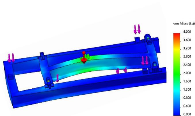
Figure 66: Testbed Assembly in Transient Configuration Under 2205 lbs. of Load
