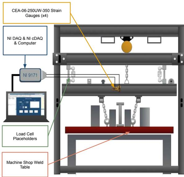
Figure 68: Structural Integrity Test Setup
