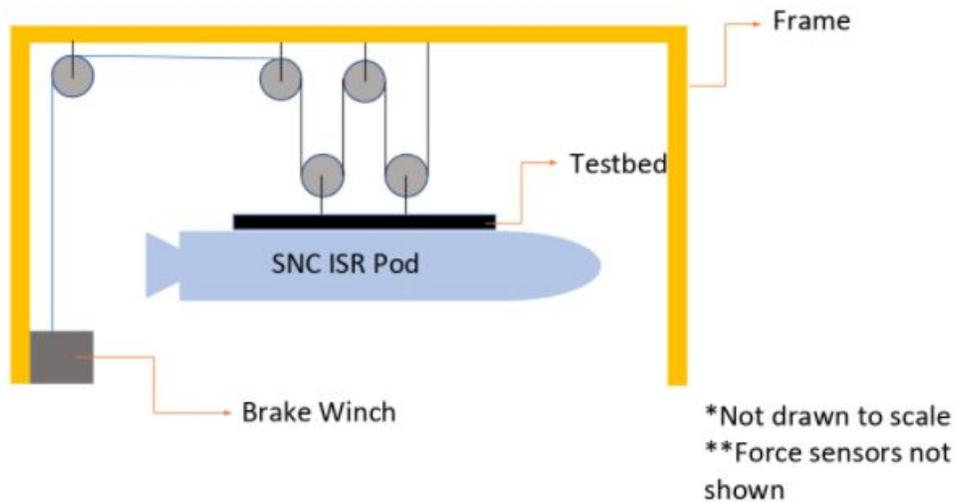
Figure 108: Pulley Lifting Mechanism on WASP
