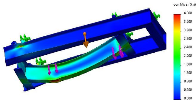
Figure 65: Testbed Assembly in Level Configuration Under 2205 lbs. of Load
