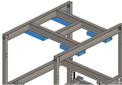
Figure 25: Forklift Slots (Blue) on the WASP Frame
