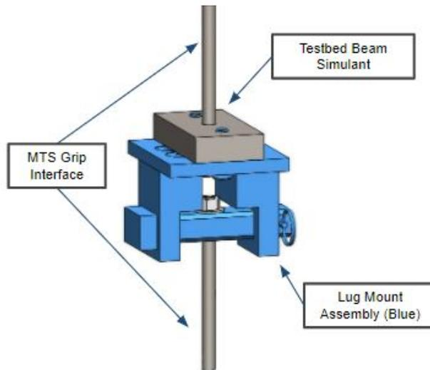
Figure 61: Clamping Setup for the LMTT
