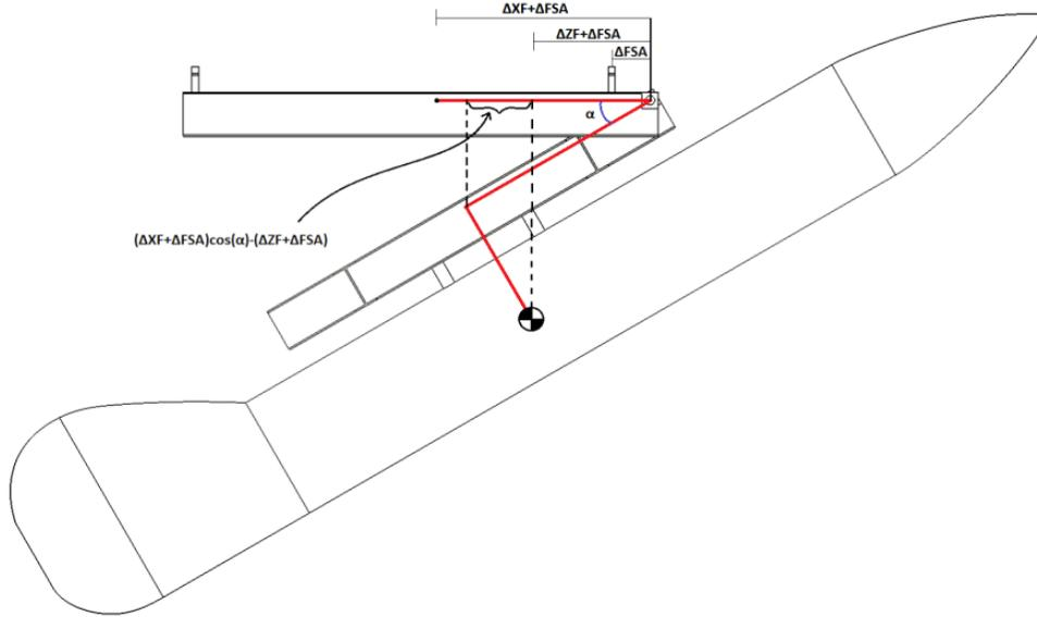
Figure 7: Pod in Tilted Configuration (for Equation Derivation)
