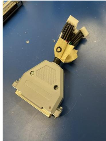
Figure 49: DAQ to Male 4-Pin Connector
