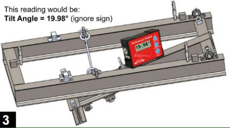
Record the TILT ANGLE of the inner testbed.
