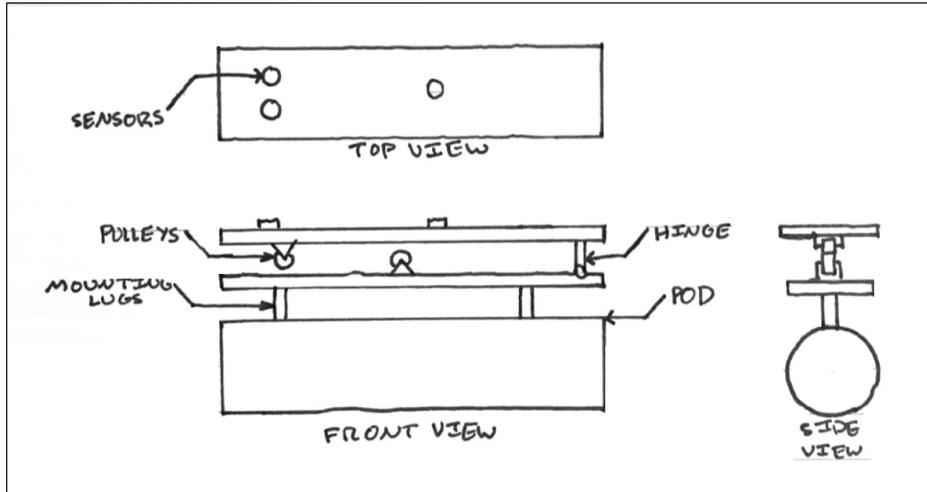
Figure 103: Indirect Connection to the Frame
