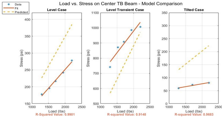
Figure 70: Structural Integrity Test Results
