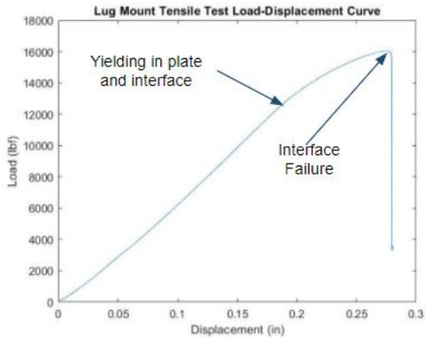
Figure 63: Force-Displacement Measurements from the LMTT
