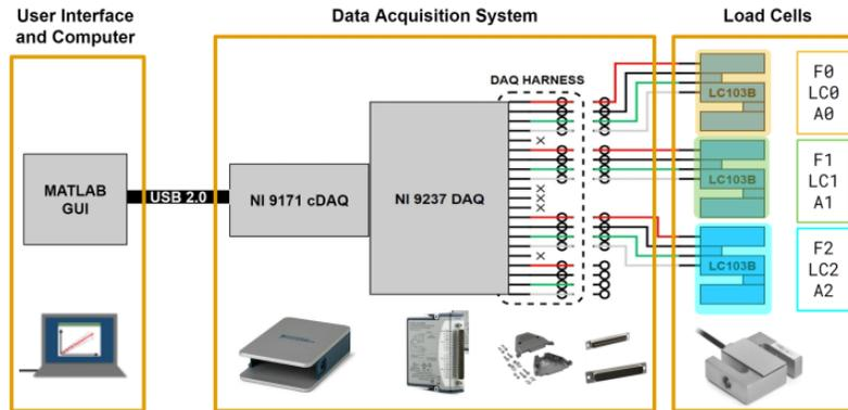
Figure 52: Electronics and Software Integration
