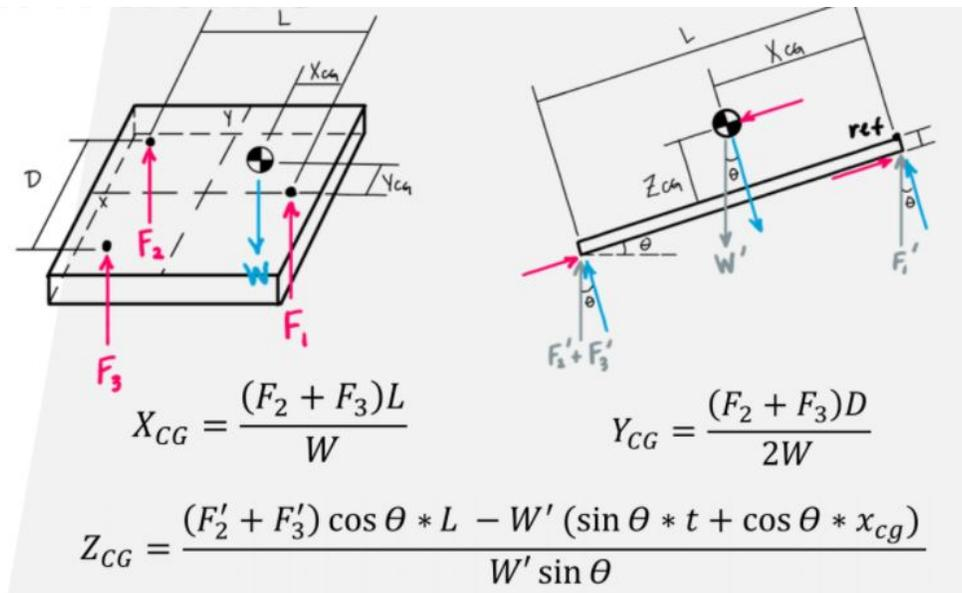
Figure 109: Generic CG Determination Equations Using Load Sensors [2]
