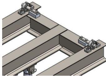
Figure 51: Inner and Outer Test Bed Connection
