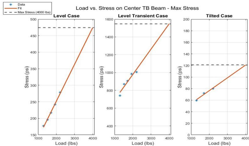
Figure 71: Structural Integrity Test Extrapolated Results
