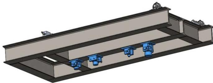
Figure 12: Lug Mounts Attached to the Testbed
