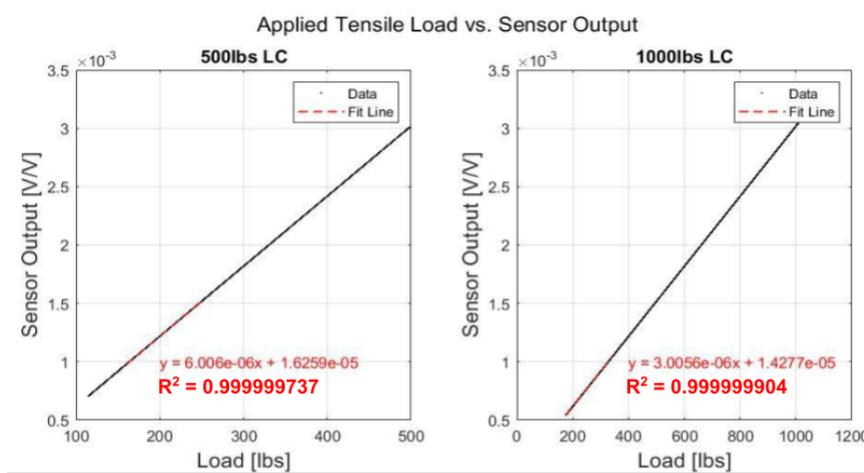
Figure 56: MTS Applied Load vs. Omega Load Cell Output Plot
