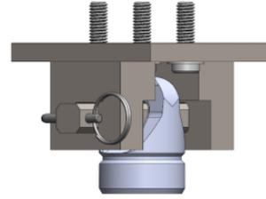
Figure 13: 100lb-Class Lug Mount with Lug Pinned    Figure 14: 1000lb-Class Lug Mount with Lug Pinned
