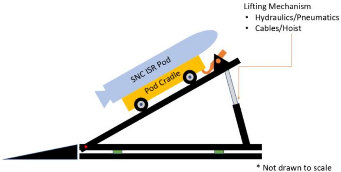
Figure 113: Cradle Platform Tilting Mechanism
