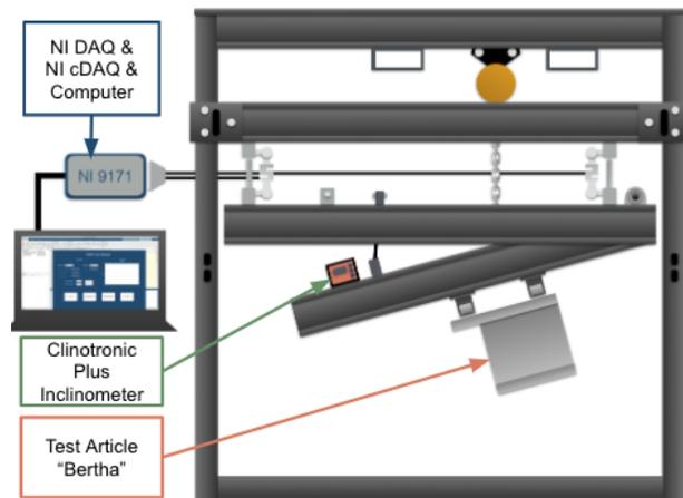
Figure 72: Measurement Accuracy Test Setup
