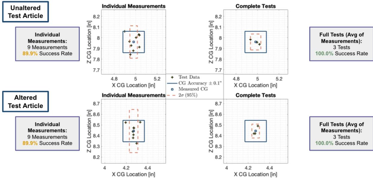
Figure 81: Predicted Range of X and Z CG Measurements for 95% of Individual Measurements and Tests
