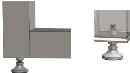
Figure 26: Leveling Feet Assembled (Left) and Transparent View (Right)
