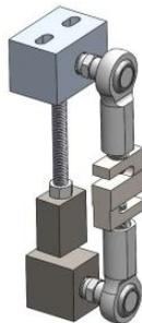
Figure 24: Force Sensor Attachment Assembly
