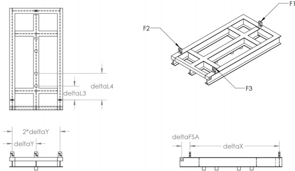
Figure 5: Load Cell Setup on Testbed
