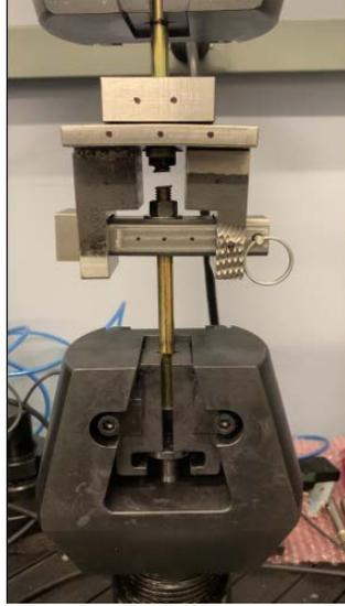
Figure 62: End of Lug Mount Tensile Test
