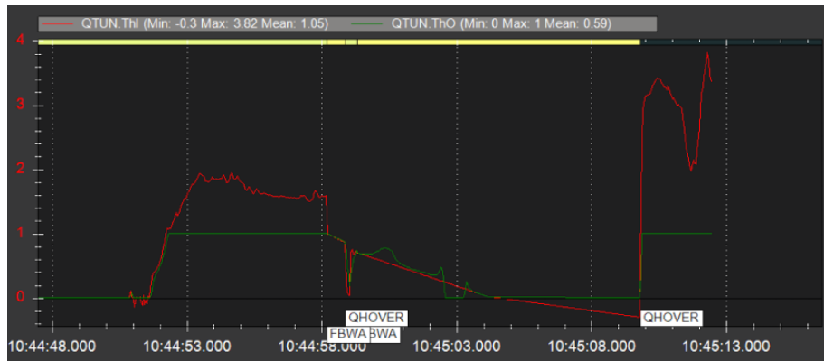
Figure 36: Hover Thrust Logs from Flight Test 1
