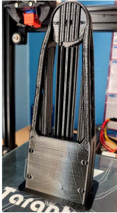
(b) Successful Rear Motor Mount Print
