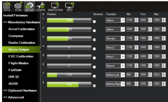
Figure 6: Controls Verification, PWM Limits Defined on GCS
