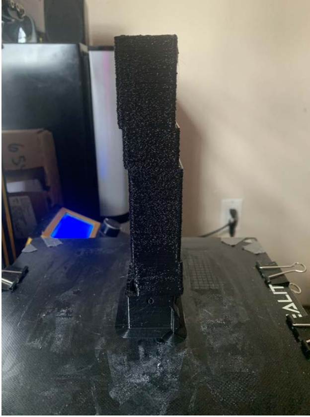
(a) Layer Shifting on a 3D Print
