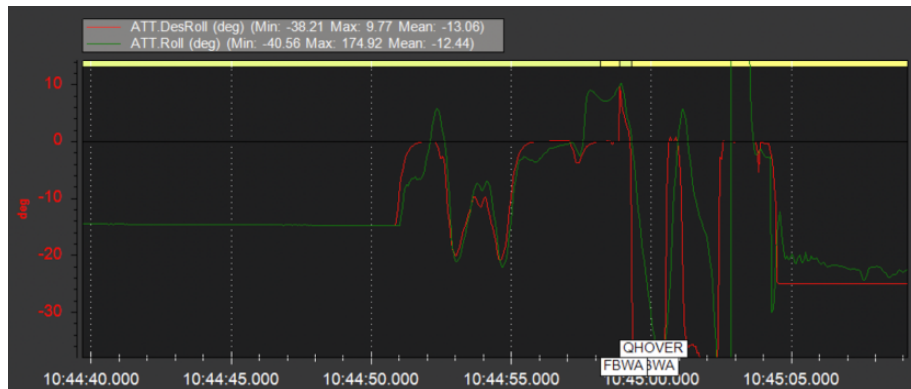
Figure 37: Desired and Actual Roll Plots from Flight Test 1
