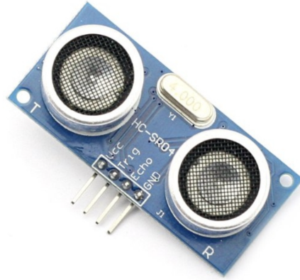
Figure 14: A Sonar Sensor [23]
