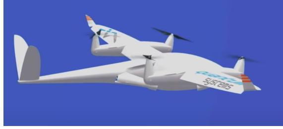
Figure 4: Quad Motor VTOL hybrid model [38]
