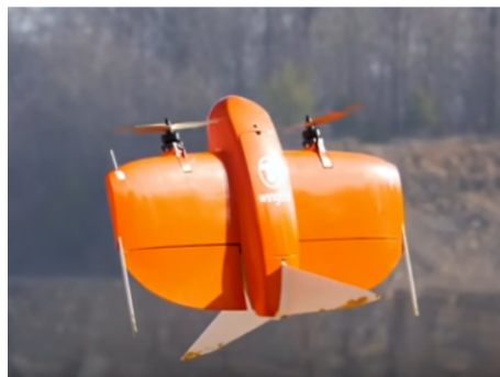
Figure 7: Dual Motor Puller Tail Sitter Configuration [15]
