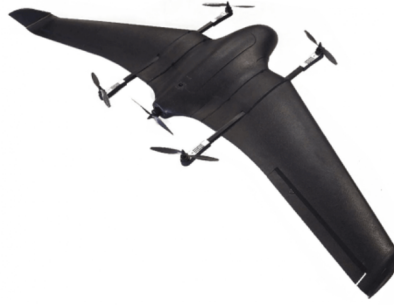
Figure 9: 4L1C Hybrid configuration [42]
