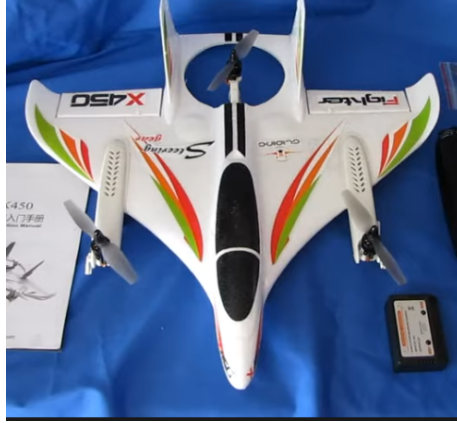
Figure 3: A tri-motor aircraft system [37]
