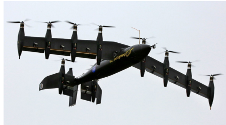
Figure 10: In Board Tilt Wing Configuration [43]
