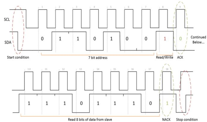
**Figure 3. Example of I<sup>2</sup>C communication** [1]
