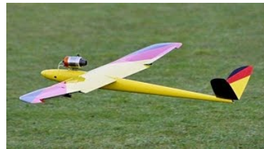
Figure 1. Application of the JetCat P90-RXi on an unmanned aerial vehicle.
