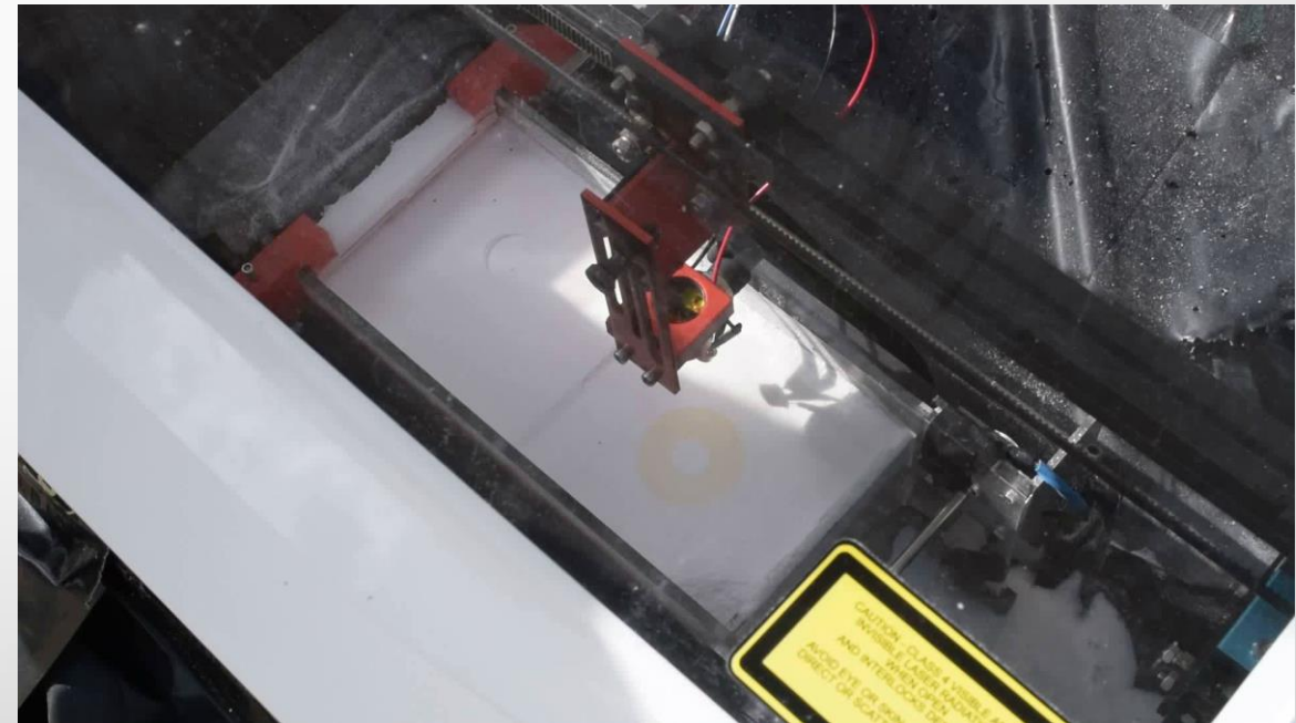
Powder Bed Sweeping New Layer of Propellant
