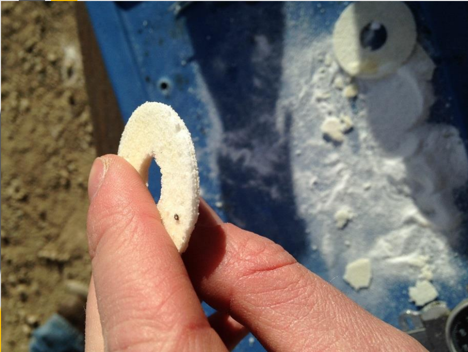
Proof of Concept – First ever 3D printed Solid Rocket Motor
