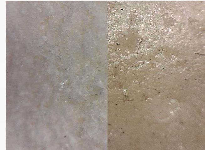
Material Comparison – printed propellant is lower quality than cast; still viable
