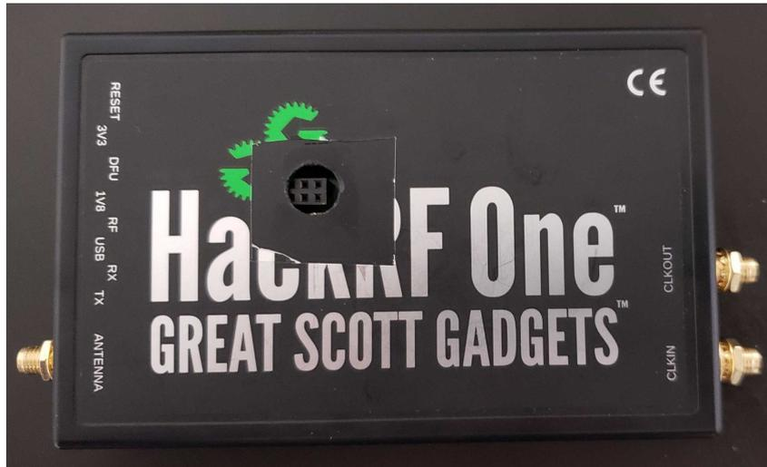
Figure 28: Hole used to access header P9 on the HackRF
