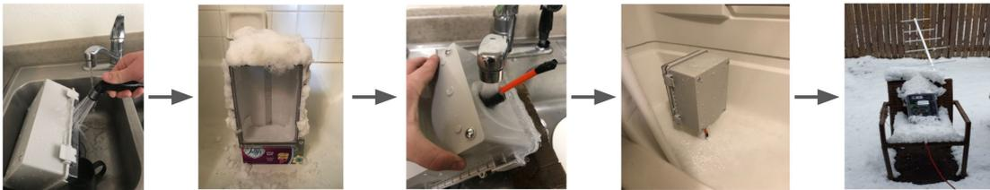
Figure 31: Water Resistance Tests Progression
