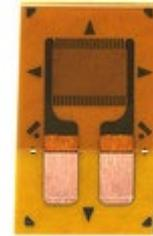
Figure: CEA-13-062UWA-350 Strain Gauge
