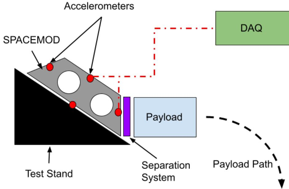
1. Place accelerometers and mount structure
