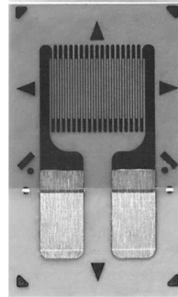
Figure: CEA-13-062UWA-350 Strain Gauge
