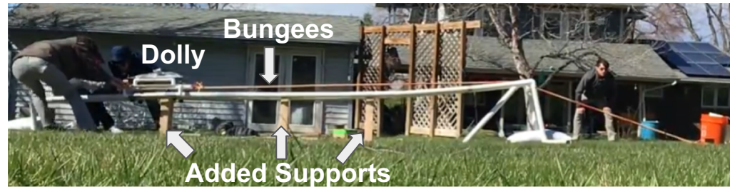
Visual representation of Launch System test set-up
