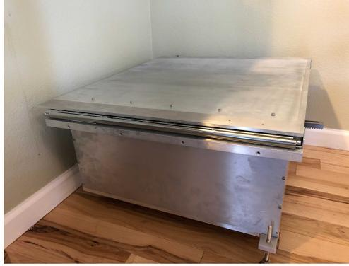
**Fig. 106 WRAITH Weather Protection Box with 6061-T6 Aluminum**
