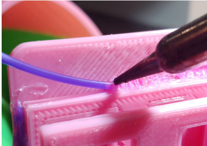
Figure 26: Welding Technique to Attach Float Structural Components
