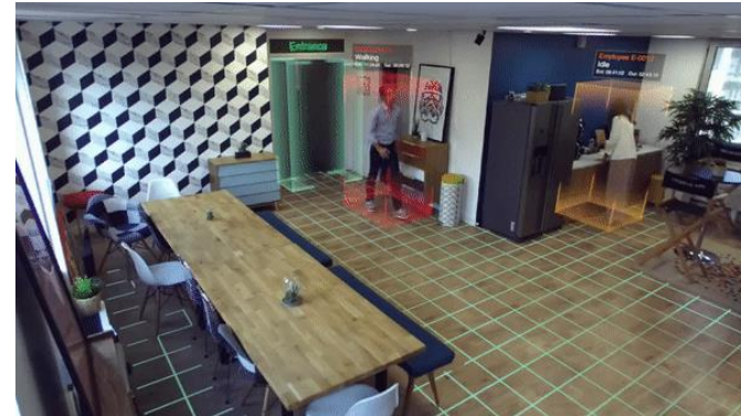
Example of ZEDs object identification and tracking capabilities.
