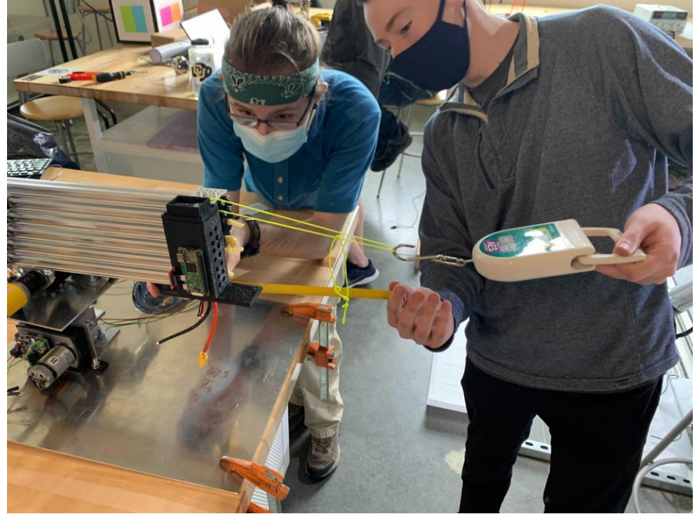
Figure 1: the horizontal test conducted by RESCUE team. Similar procedure was done for vertical
