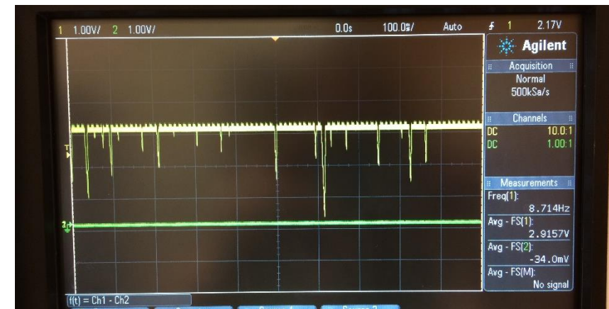
Issue Encountered after Testing – Signal not square
