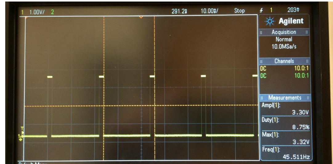
Full Throttle: 8.75% Duty Cycle (1.92 ms pulse)
