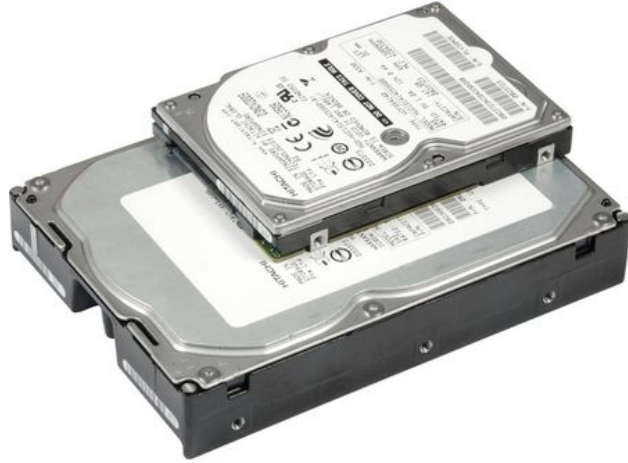
Figure 35: 2.5 inch and 3.5 inch form factor hard disk drives [45].
