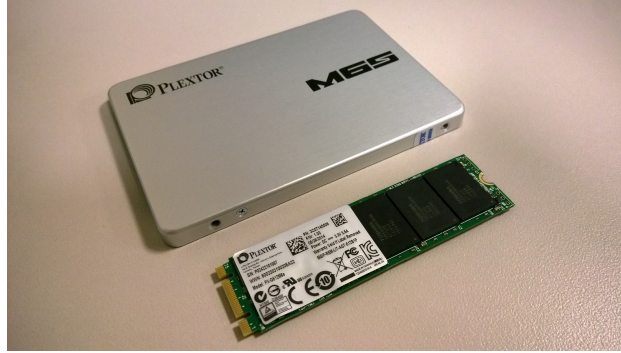
Figure 36: 2.5 inch drive and M.2 interface drive [46].
