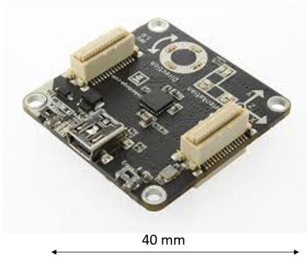
Figure 39: A typical inertial measurement unit [18].
