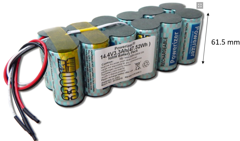
Figure 28: A multi-cell configuration of NiMh batteries [54].
