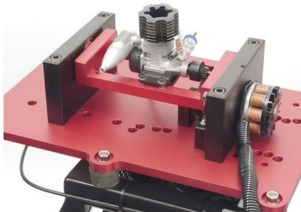
Figure 33. Dynamometer test setup
