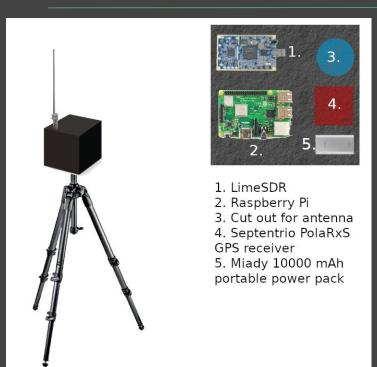
Each transmitter and receiver will feature a casing for the electronics that will hold the LimeSDR, Raspberry Pi, a battery pack, and space for wiring and a connection to the antenna. The electronics casing will be thread-mounted to a camera tripod.
