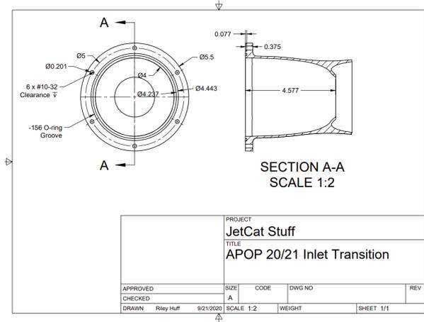
Figure 13: AFRL Engine-Inlet Adapter
