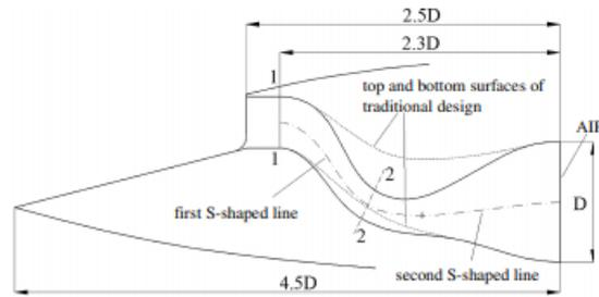
Figure 11: Example of Converging-Diverging Inlet
