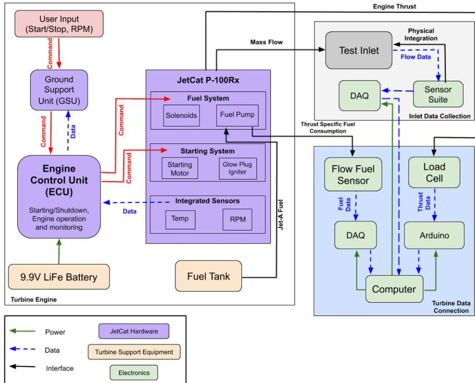
Figure 5: JetCat Turbine Engine FBD
