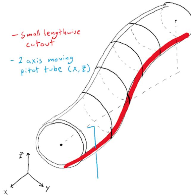
Figure 19: Slotted Pitot Tube Isometric View
