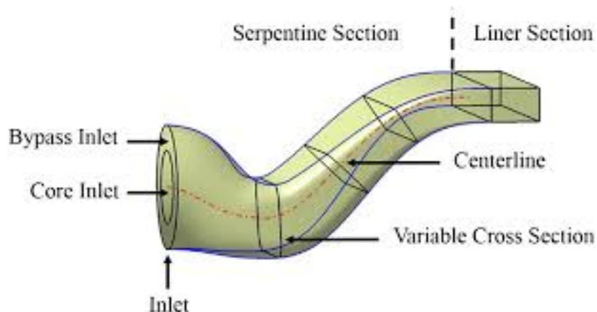
Figure 9: S-Duct with a non circular bypass inlet cross section
