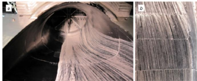
Figure 18: Surface Oil-Flow Visualization
