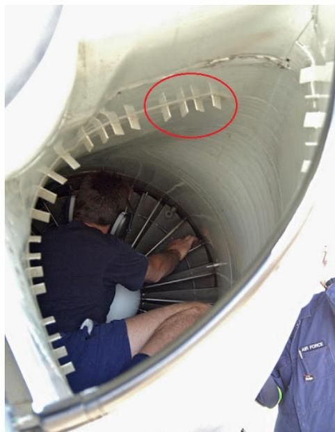
Figure 6: Example of Vortex Generator on F-111 Inlet
