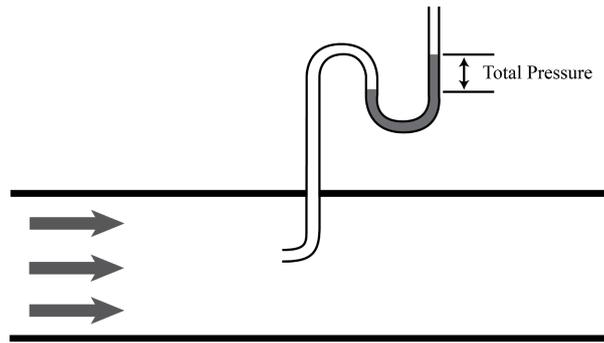
Figure 14: Pitot Probe Cross-Section
