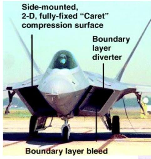
Figure 8: Example of an F-22 Inlet
