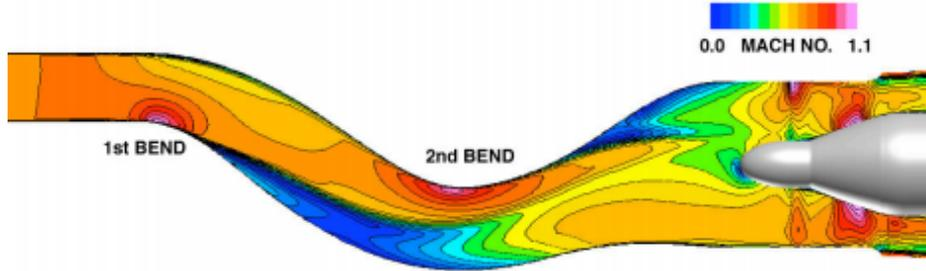
Figure 1: Illustration of Flow Inside an S-Duct
