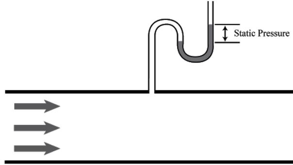
Figure 16: Static Pressure Port Cross-Section
