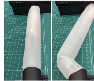
Figure(3): failure due to Buckling (horizontal loading) Figure(4): failure due to bending (yielding) (vertical loading)
