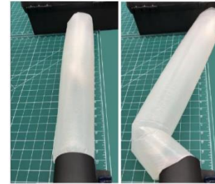
Figure(3): failure due to Buckling (horizontal loading)
