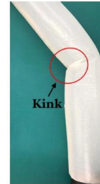
Figure 2: failure due to bending (yielding) (vertical (perpendicular) loading)
