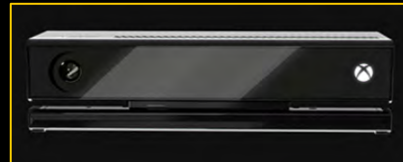
Microsoft Kinect V2: 2D (RGB), 3D (IR) image capture
