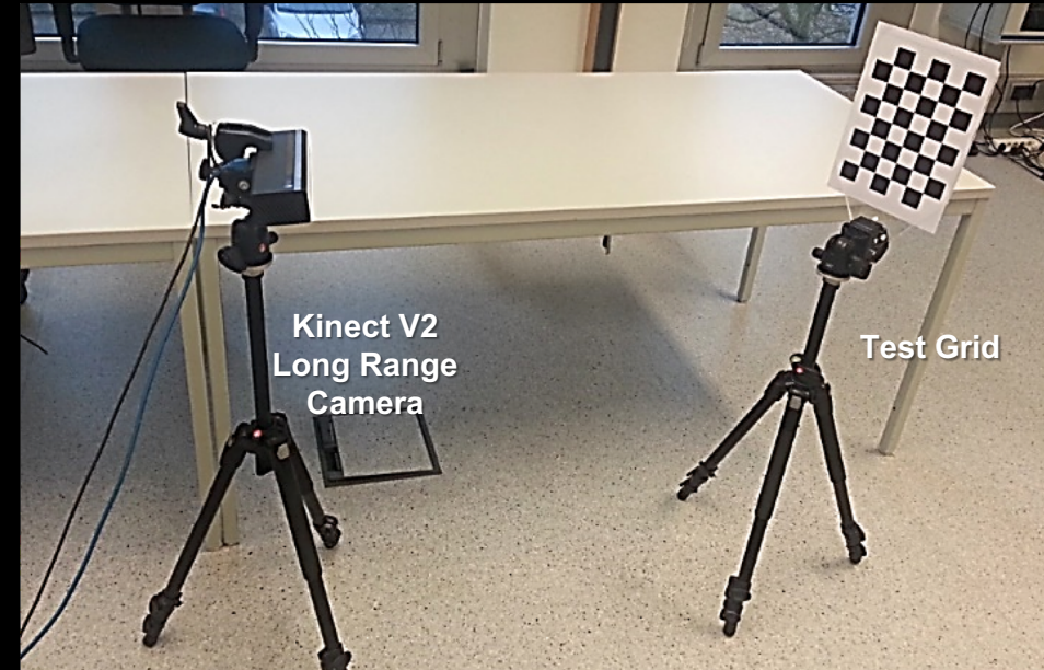
Fig 14: Example of calibration testing setup
