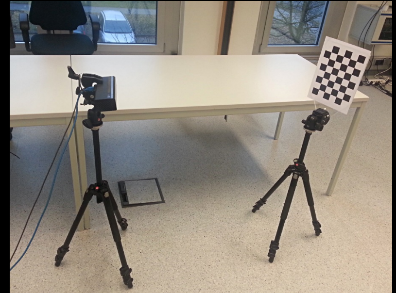
Fig #: Example of calibration testing setup
