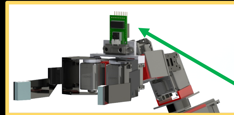
Short Range RGB Camera & Prox Sensor on Robotic Arm Wrist
