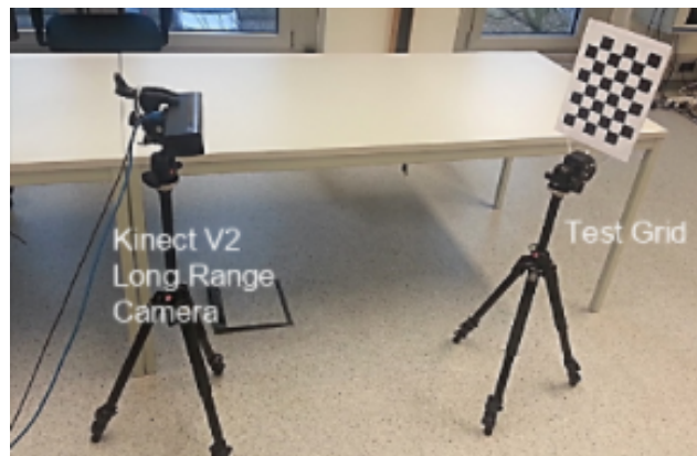
Fig. 4 Test setup to find error in the Kinect V2 depth sensor.
