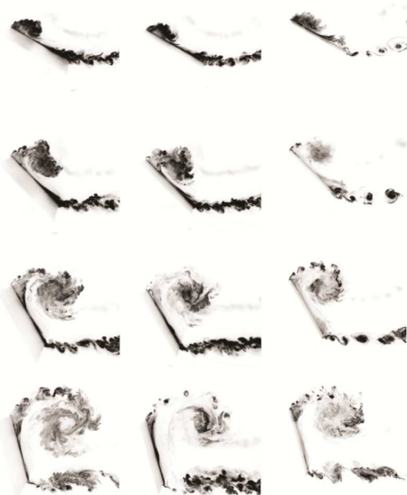
Figure 1: Dye flow visualization of a rectangular panel undergoing a pitch motion. Granlund et al. (2013) J. Fluid Mech.
