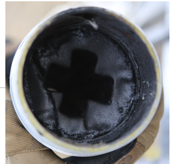
Pyrolyzed fuel grain post test
