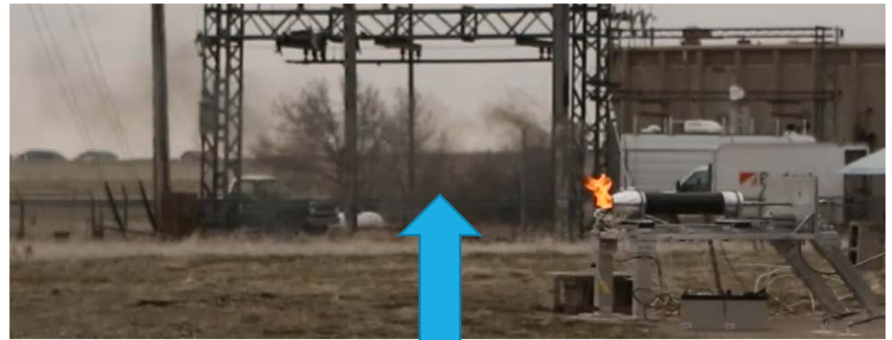
Black smoke viewed during pre-combustion due to burning of fuel
