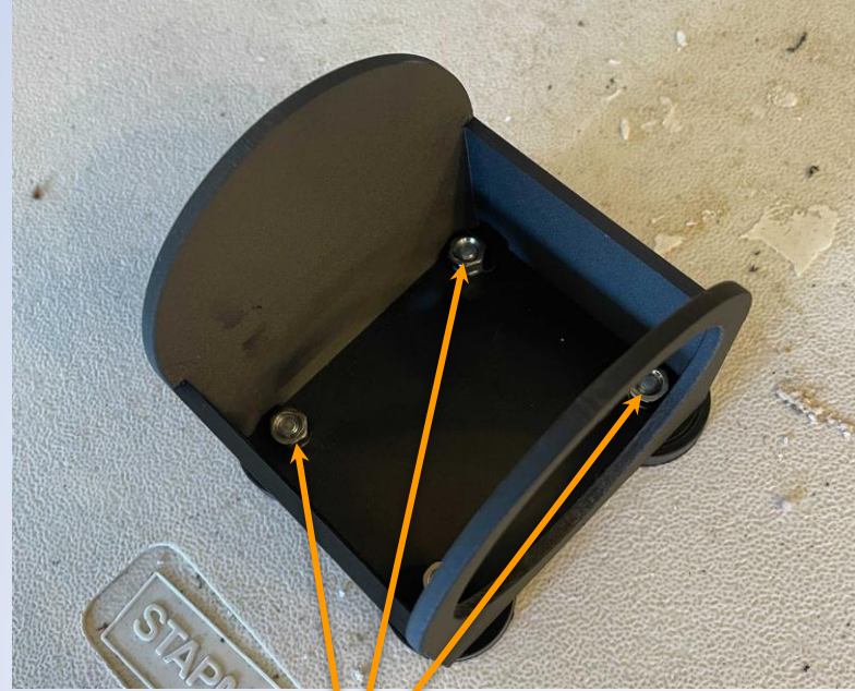
Bolts (5 mm x 9.5 mm) Integrated with Magnets
