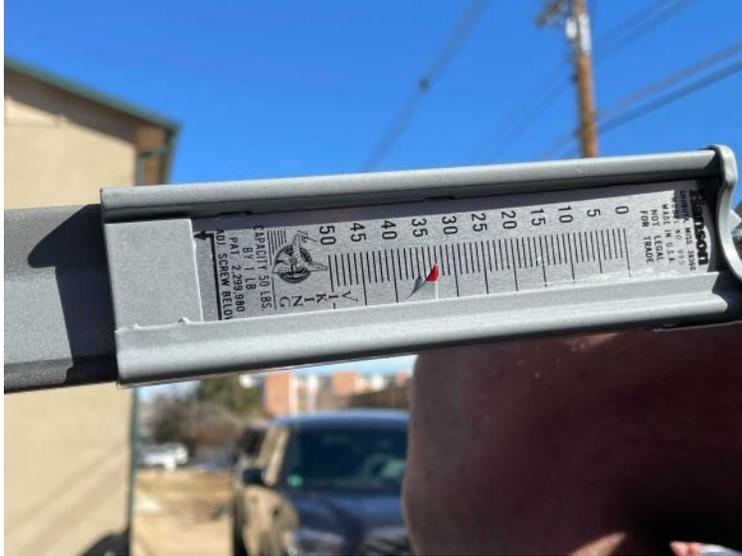
Figure 25: Pull Test Force Measurement
