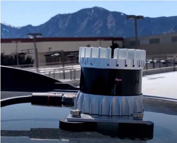
Figure 15: Manufactured Aluminum Mount (New Configuration)
