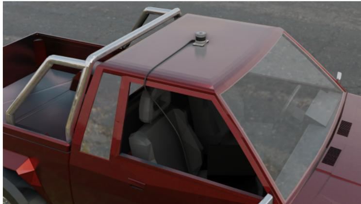
Figure 8: LiDAR Mounted atop the Mission Vehicle
