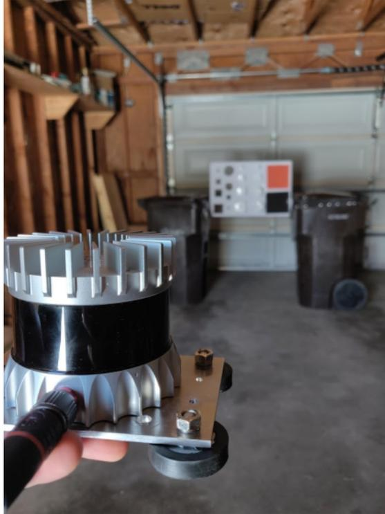
Figure 27: Small Scale LiDAR Test Setup (Actual)
