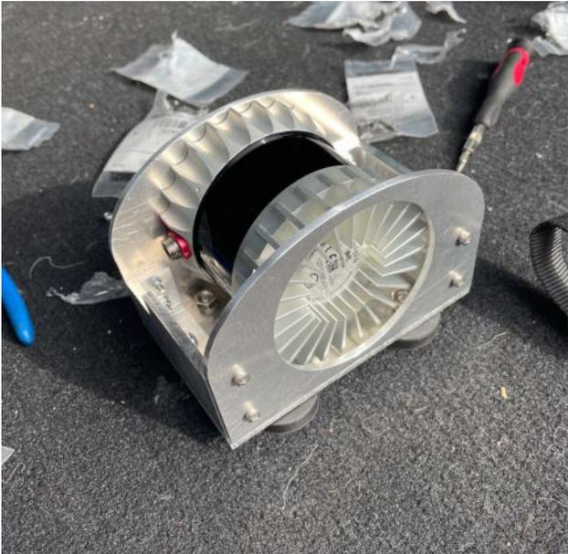
Figure 14: Manufactured Aluminum Mount (Old Configuration)
