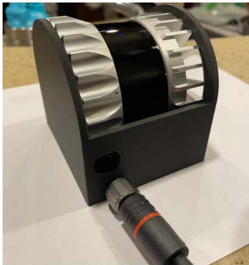
Figure 11: 3D-Printed Nylon/Carbon Fiber Composite Fit Check Mount
