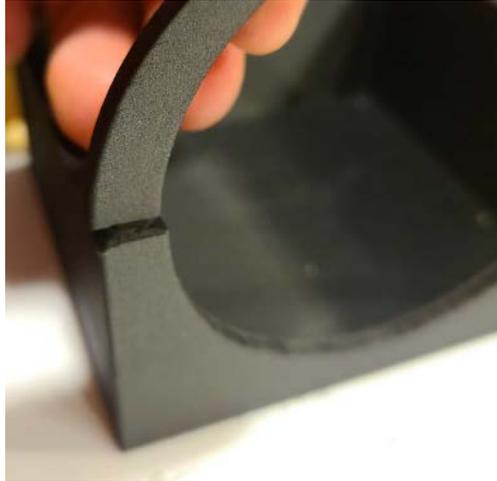
Figure 12: 3D-Printed Nylon/Carbon Fiber Crack
