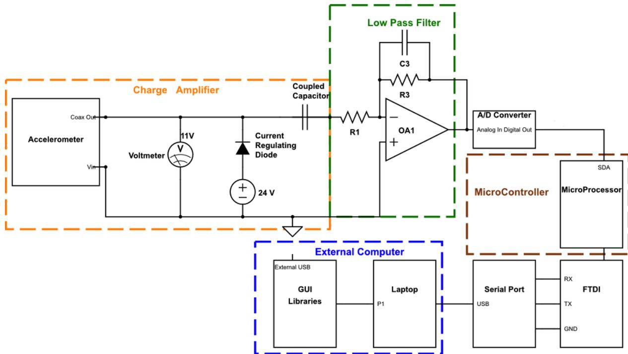
Figure 4.12: Circuit Diagram for Single Microcontroller Design
