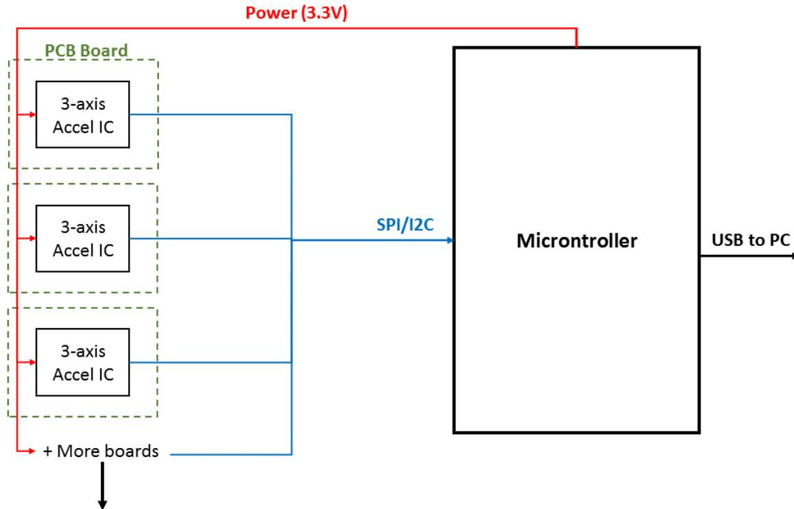
Figure 4.9: Digital Output Accelerometers Design Option Configuration
