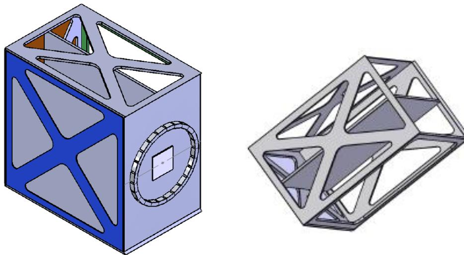
Figure 4.2: Mass Reduced Paneled Box Structure
