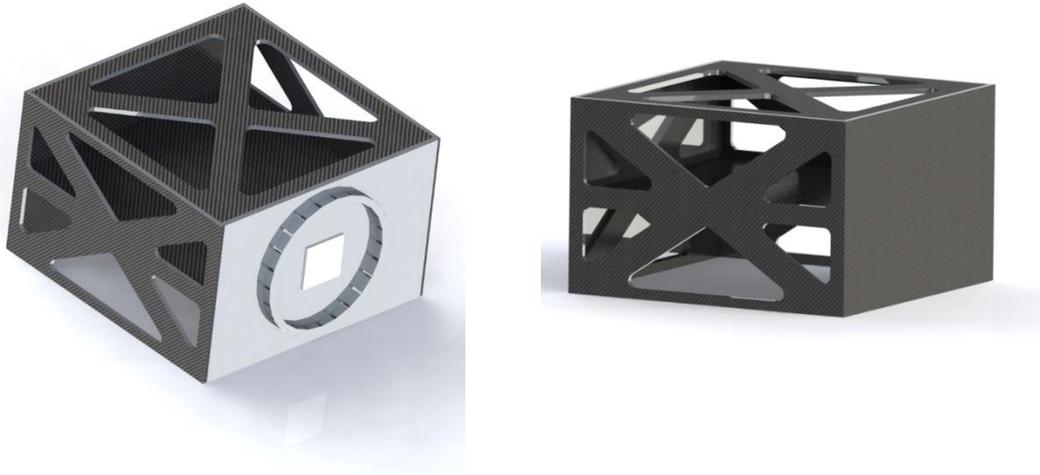
**Figure 4.4: Rendering of proposed sandwich structure with weight-relieving cutouts**
