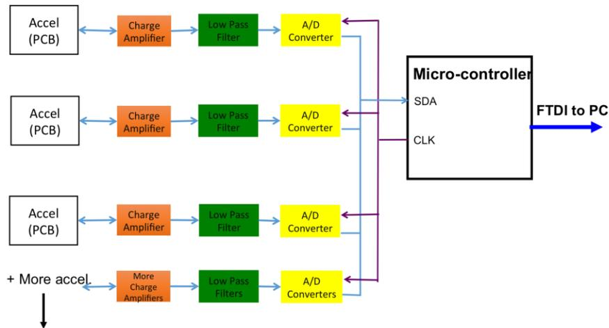
Figure 4.11: Build Data Acquisition System with One Micro-Controller
