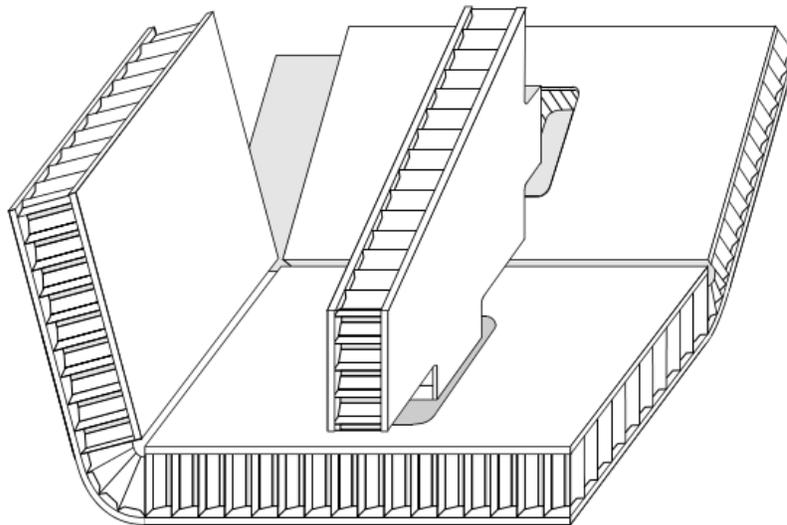
**Figure 4.5: Concept drawing of folded-panel construction<sup>1</sup>**
