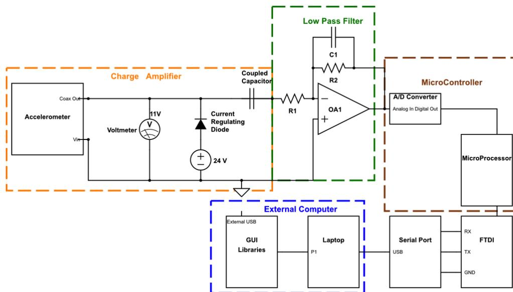
Figure 4.14: Circuit Diagram for Multiple Micro-Controller Configuration
