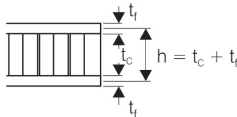
**Figure 4.6: Definitions of honeycomb geometry terms**
