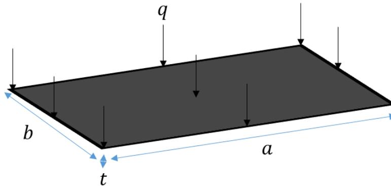
**Figure 4.3: Flat plate showing uniform pressure distribution ( $q$ ) and plate dimensions**
