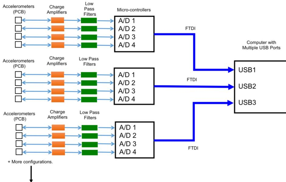
Figure 4.13: Design with Multiple Micro-Controllers
