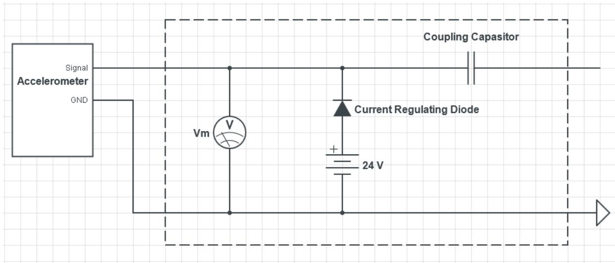
**Figure 4.10: Charge Amplifying Circuit**
