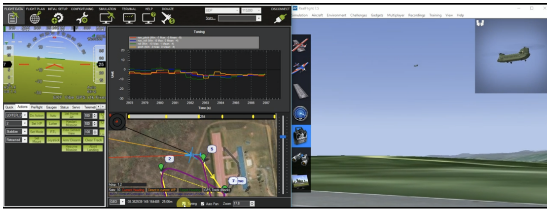
Figure 42: SITL simulation in APM Planner with Chinook Helicopter
