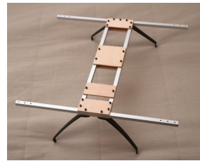
Figure 13: H-Shaped Quadcopter Frame
