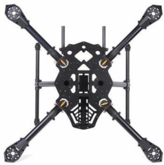
Figure 12: X-Shaped Quadcopter Frame
