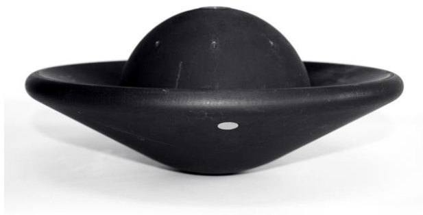
Figure 13: NASA's MMEEV designed to return samples from space to Earth. MMEEV is designed to puncture the atmosphere at high speeds before impacting the surface of Earth. [14]
