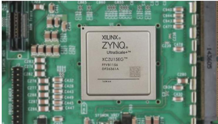
Figure 17. Xilinx Zynq UltraScale+ MPSoC kit
