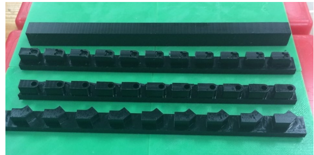
Fig. 17 Raw Delrin Bars Converted to Part Blanks
