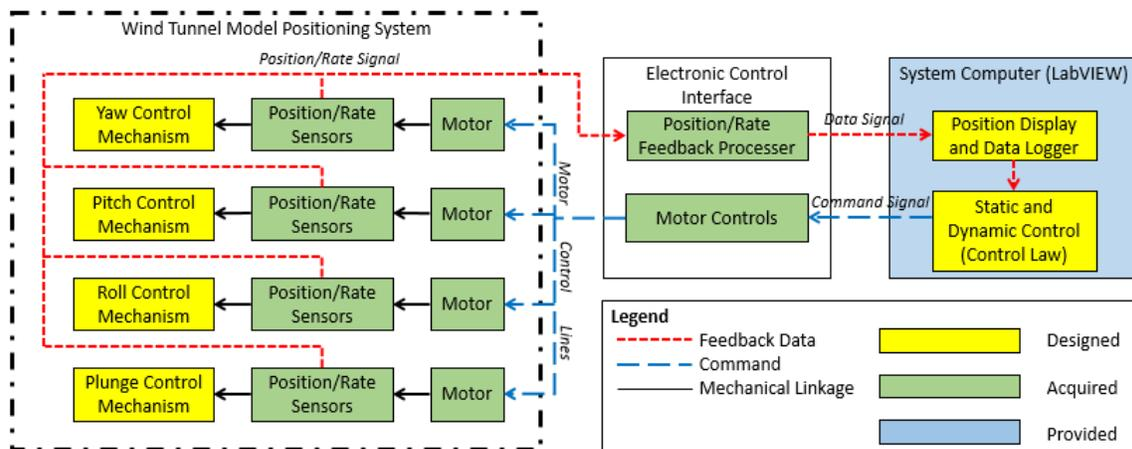
Figure 3. Functional Block Diagram for Wind Tunnel Model Positioning System
