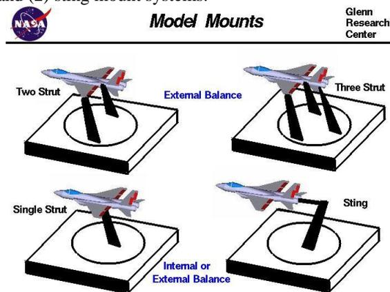
Figure 1. Typical mechanical positioning systems <sup>4</sup>
