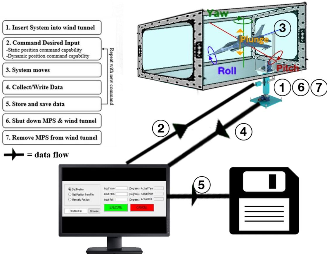
**Figure 2.** CONOPS for complete wind tunnel system
