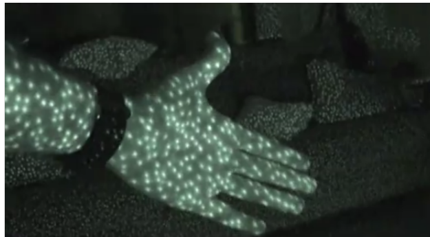
Figure 23 Depth Sensor Infrared Dots on a Hand
