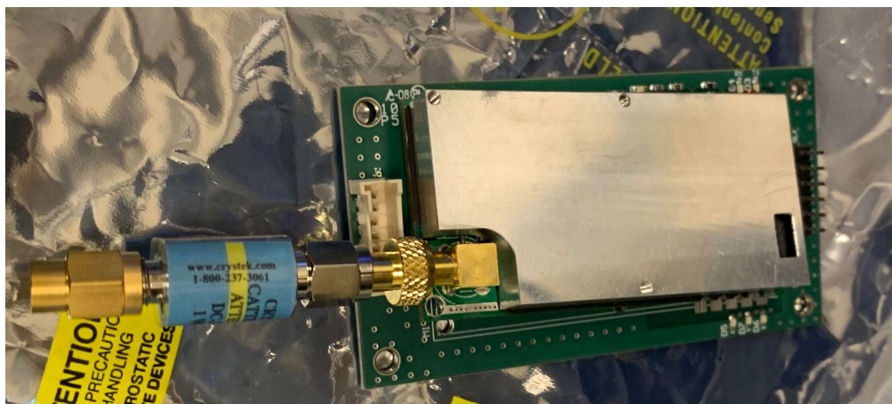
Figure COMM-5: UHF Backplane revision 1 integration
