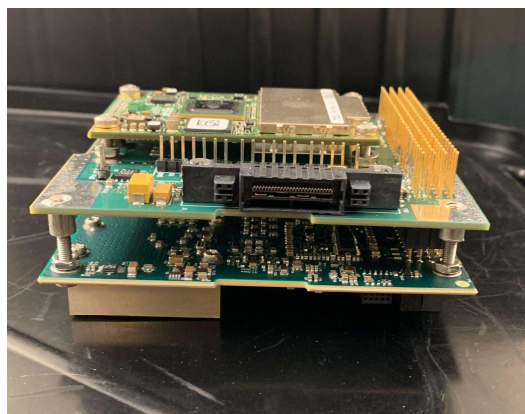
Figure COMM-6: S-band Daughterboard revision 1 integration
