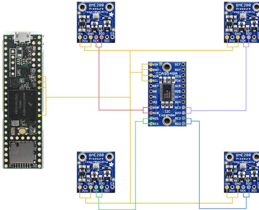
Figure 4. FADS Bay Circuit Diagram
