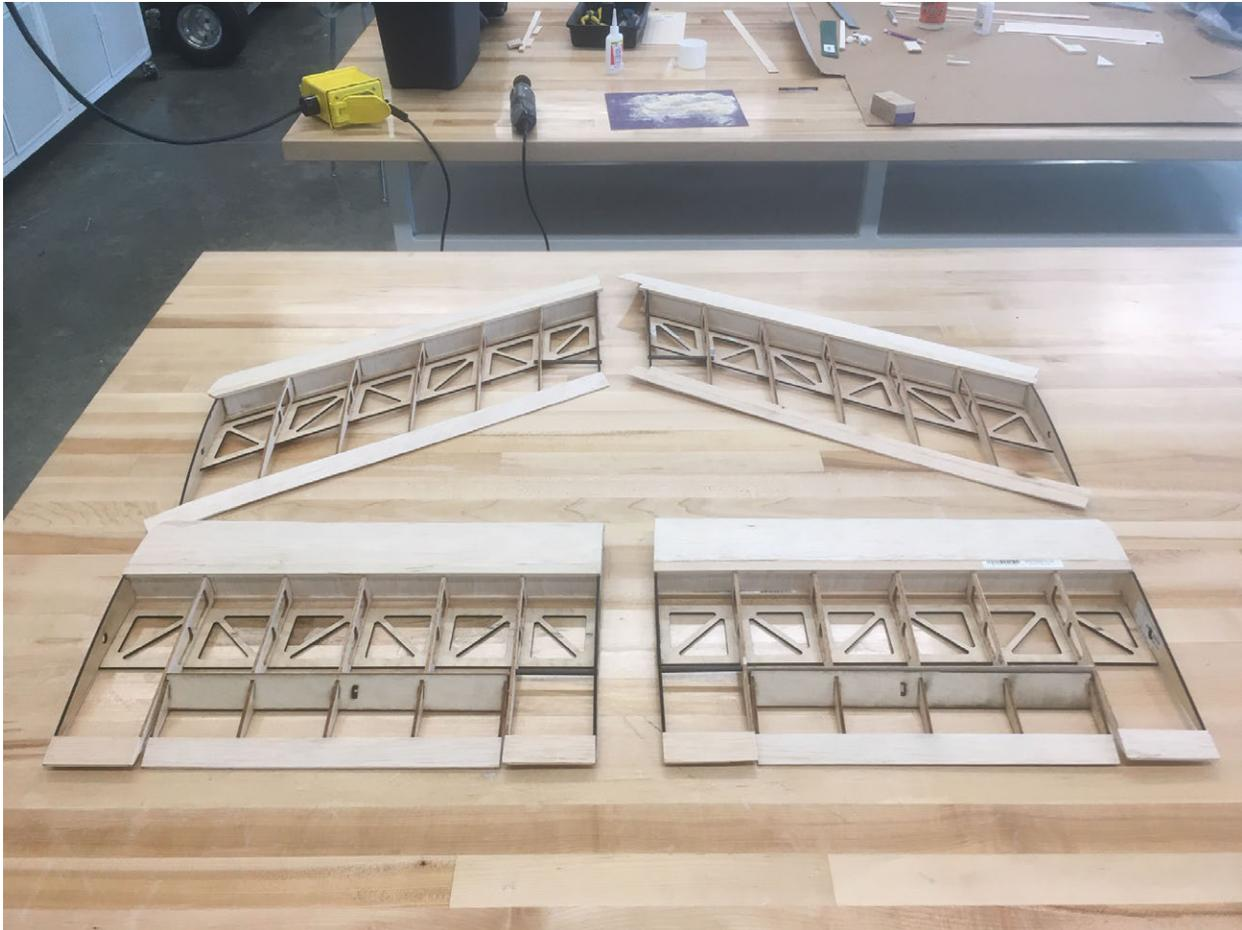
**Figure 9. Wing sections showing bays used for airframe integration of various subsystem components as well as integrated elevons**
