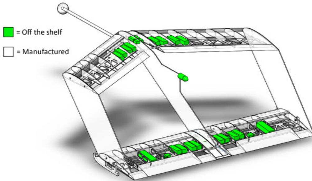
Figure 6. Manufactured and Off the Shelf Components
