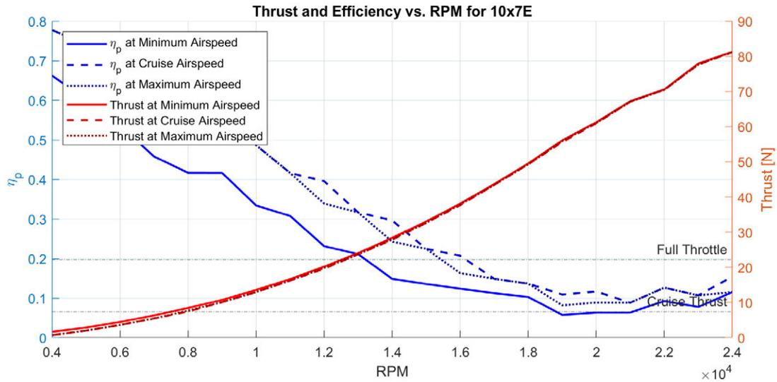
Figure 19. Example of Predicted Thrust and Efficiency
