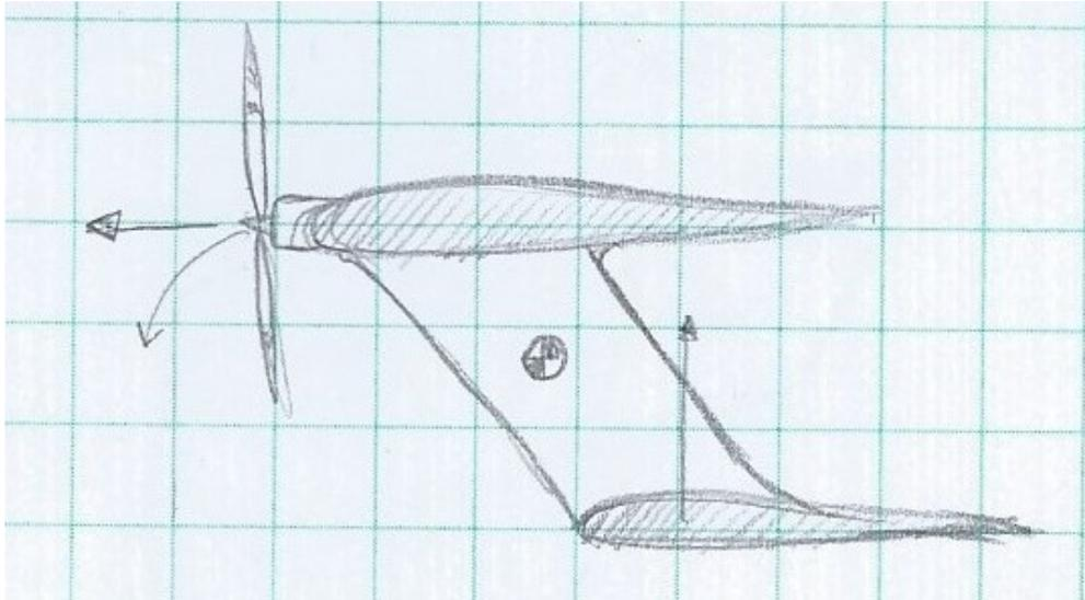
Figure 65. Puller Configuration, Side View
