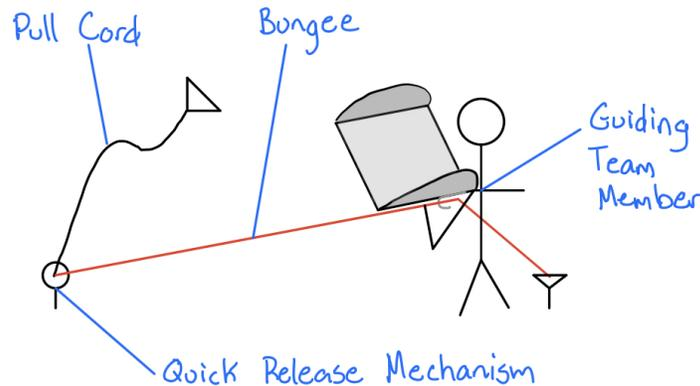
Figure 70. IRISS Hand-Bungee Diagram
