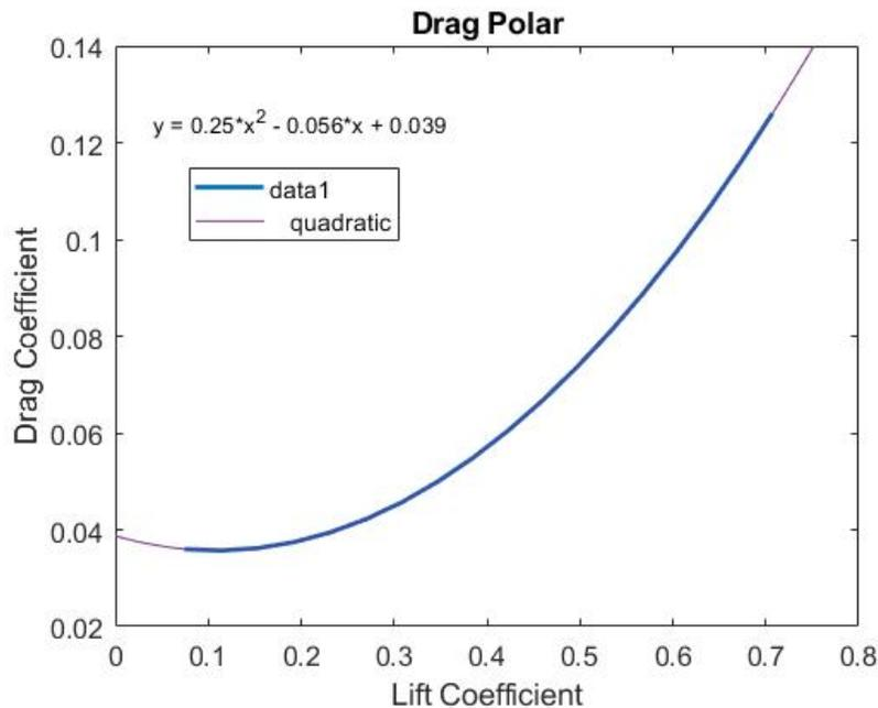
Figure 32. AVL Calculated Drag Polar
