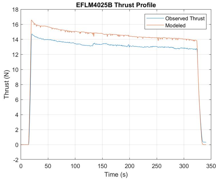
Figure 22. Thrust Profile Comparisons
