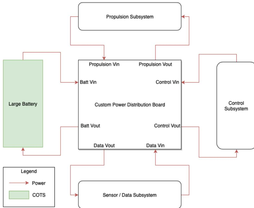
Figure 60. Power Configuration Diagram
