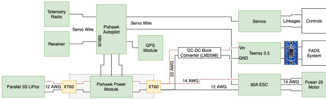
Figure 3. Overall Electronics Circuit Diagram
