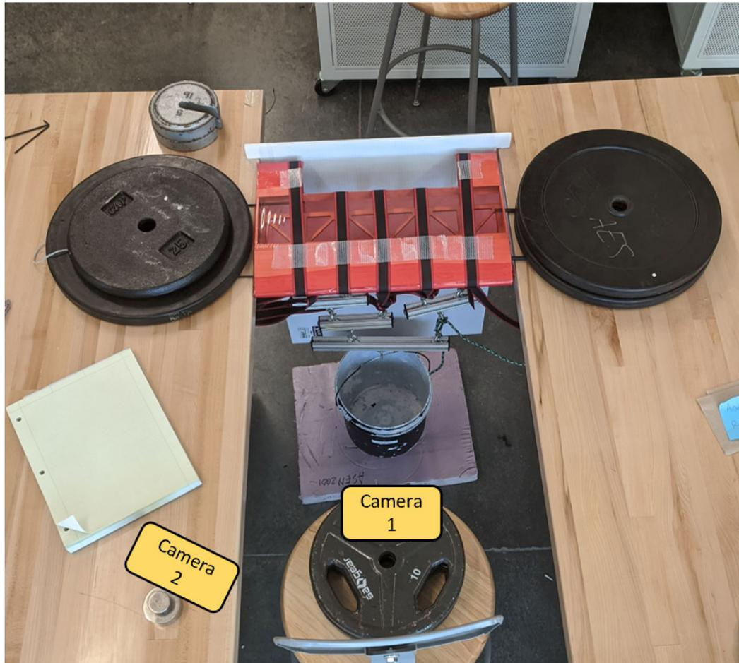
**Figure 16. Whiffletree Setup**
