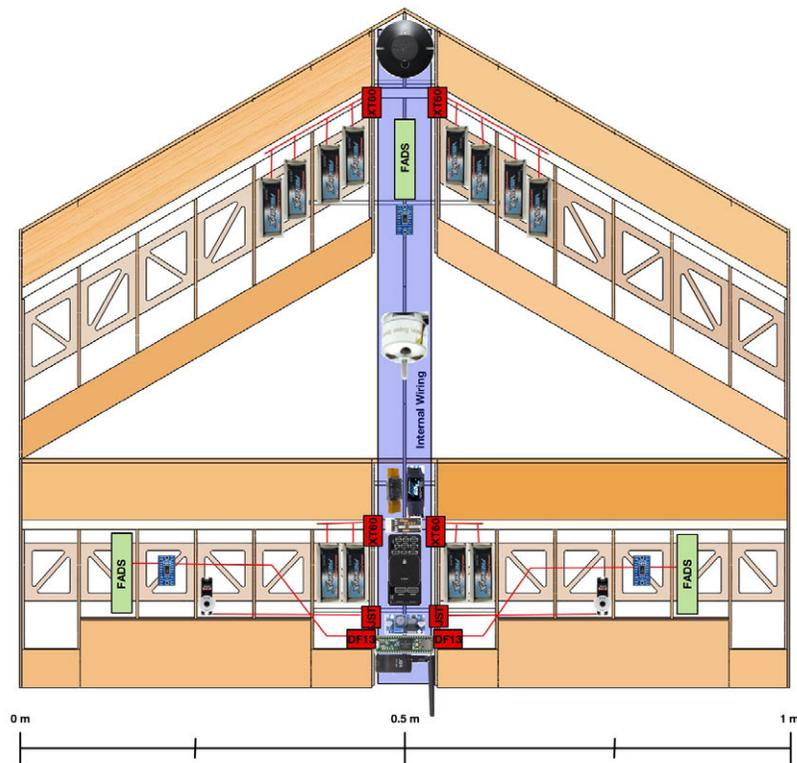
Figure 7. Aircraft Circuit Integration Layout
