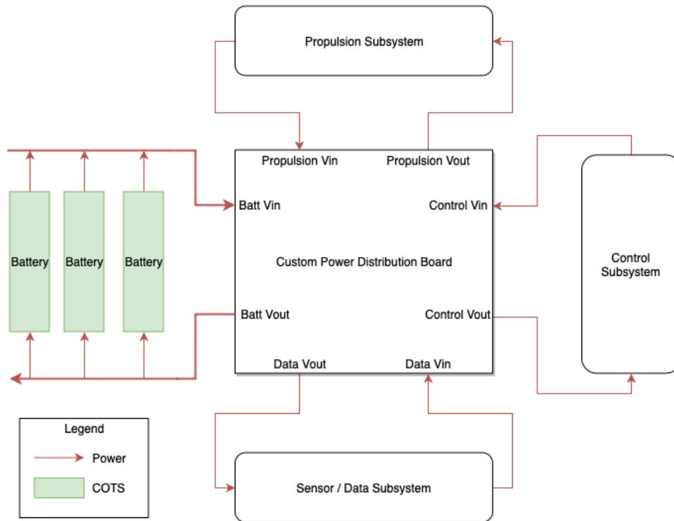
Figure 61. Power Configuration Diagram
