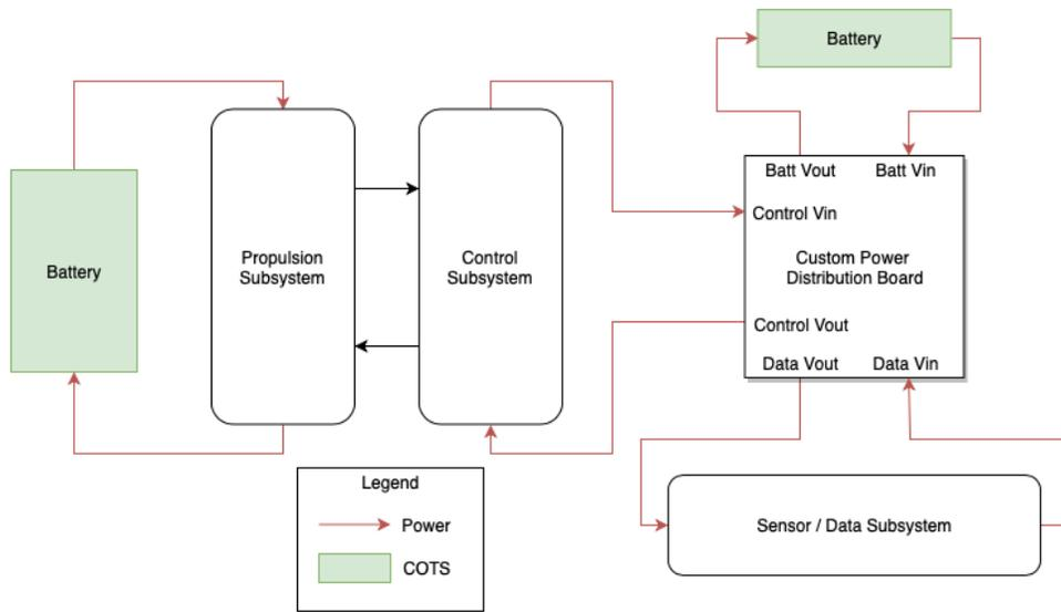
Figure 62. Power Configuration Diagram
