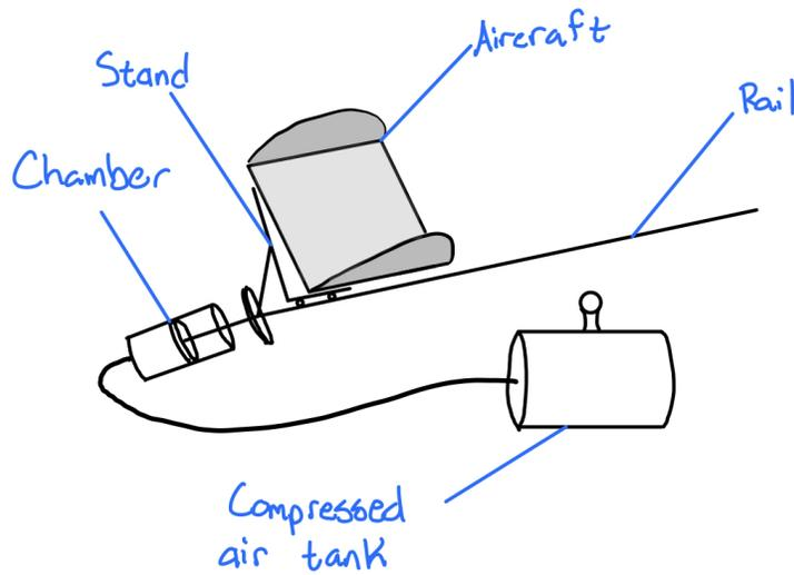
Figure 72. Pneumatic System Diagram
