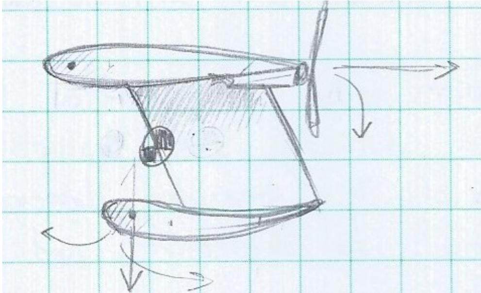
Figure 64. Double Pusher with Reflexed Wing, Side View
