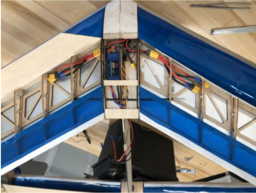
**Figure 11. Power and Electronics Integration**
