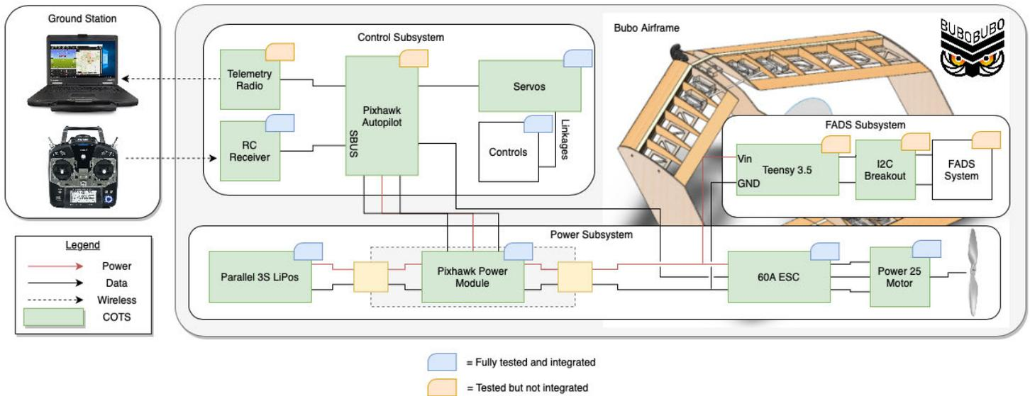
Figure 2. Functional block diagram of BUBO BUBO with integration status at cutoff
