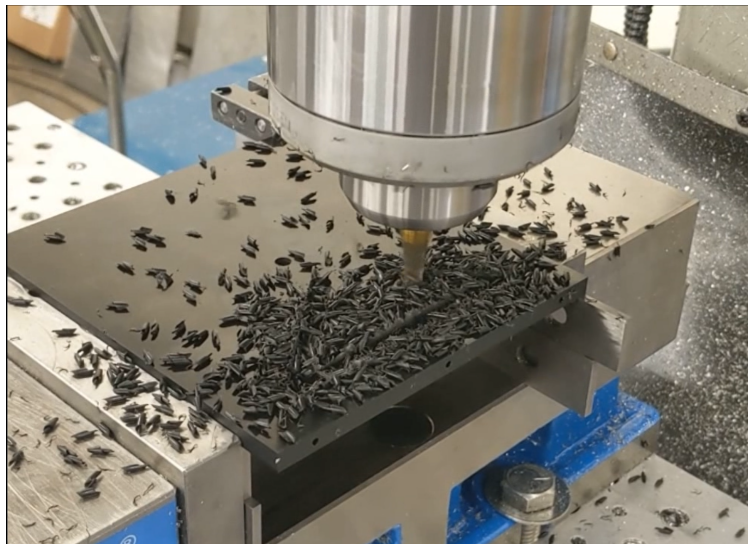
Figure 31: Picture of a Wall Section on the CNC Mill
