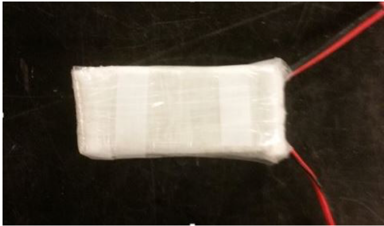
Figure 5. Insulation Configuration around a Battery
