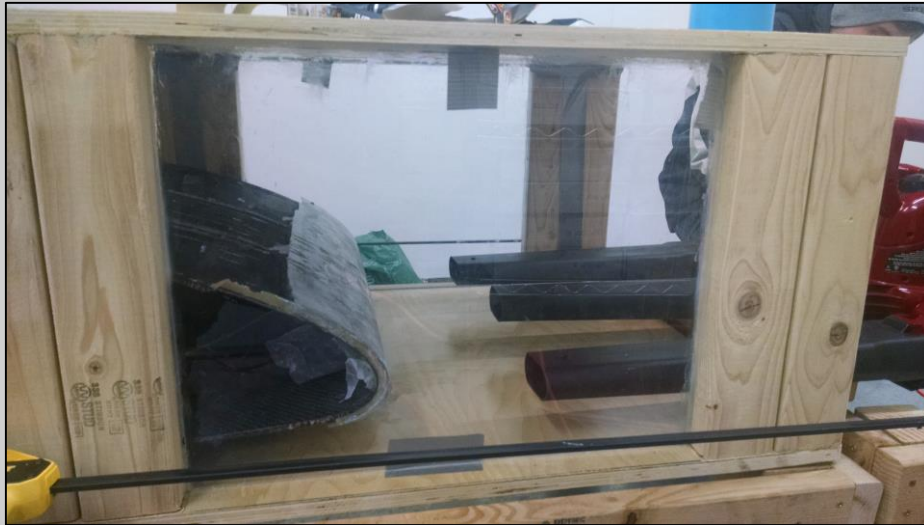
Wind cage, wind speed, test section setup in walk-in freezer
