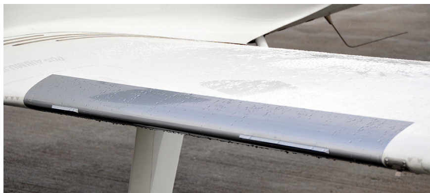
Figure 8. Thermo-electric heating elements implemented on general aviation aircraft. 2
