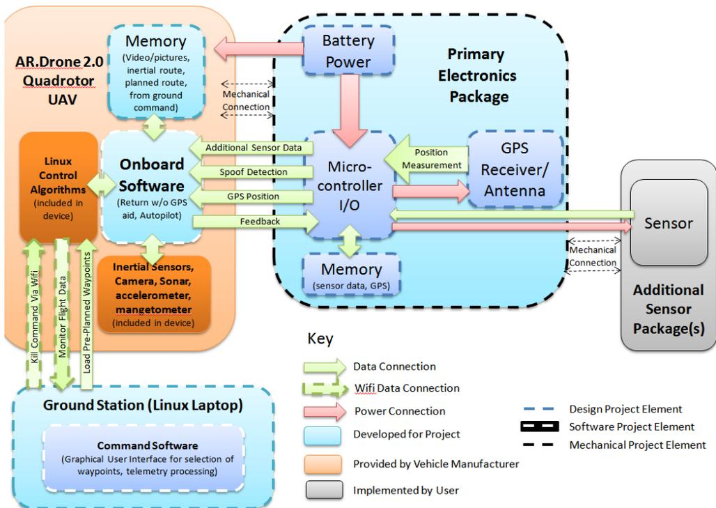
Specifically, the user will program the vehicle's route using the graphical user interface (GUI) at the ground station. This GUI will provide a map of surrounding areas and allow the user to select the desired GPS waypoints. Once the route is selected, the ground station will upload the route to the vehicle using a Wi-Fi connection. The vehicle will then act autonomously, using onboard GPS to fly
