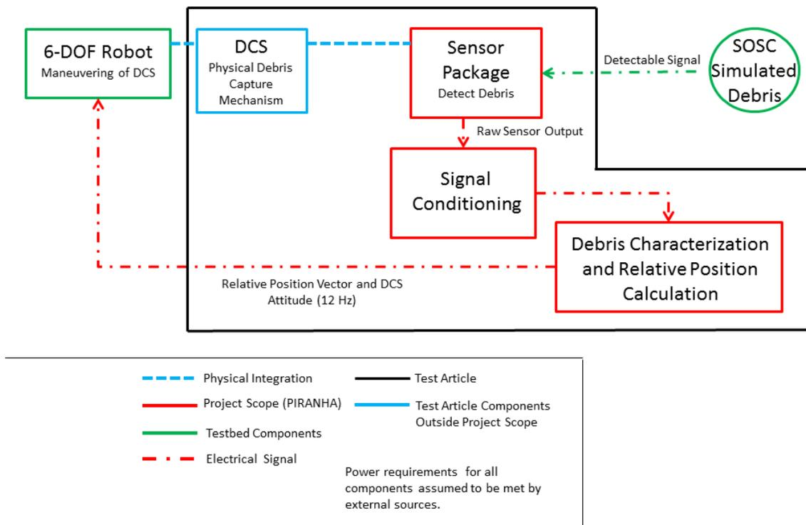
**Figure 2: Functional Block Diagram of PIRANHA**
