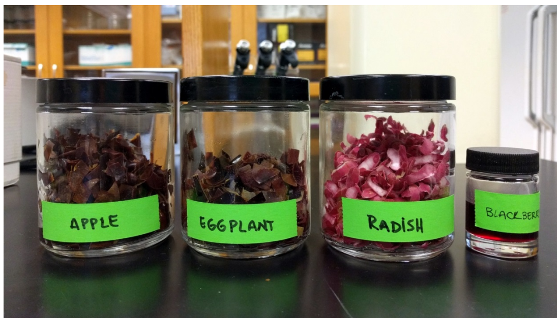
Figure 2. Skin samples for apple, eggplant and radish, and extraction solution for blackberry after filtering. Notice that the skin samples have little to none fruit flesh (white).
