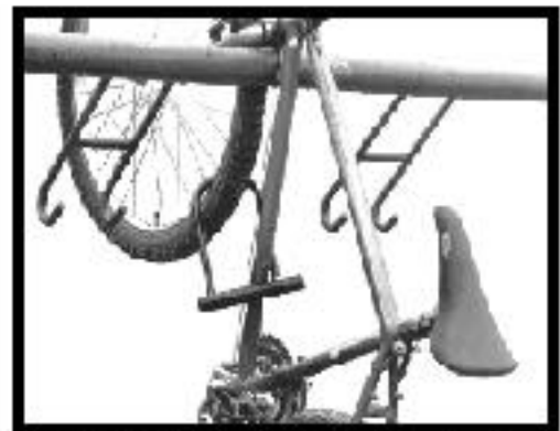
WRONG: This bike is only locked to itself, and not to the bike rack! If the front wheel is released, the bike can be removed from the rack.
